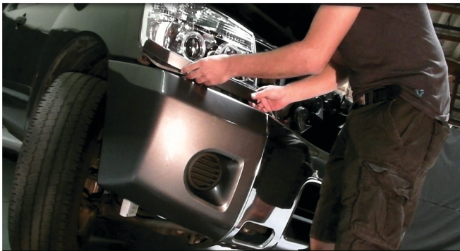
13) Reinstall Headlight Trim Panel by pushing it gently into place, being sure to install it fully so that the trim panel is secure.
