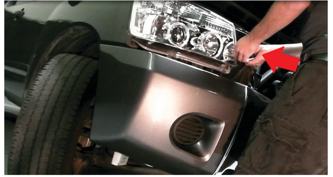
12) Connect SPYDER headlight wiring harness to the truck's wiring harness.
