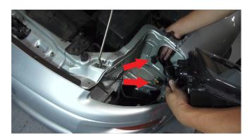
2) Once the bolts have been removed, you will need to remove the headlight harness connected to the OEM headlamp, shown here. Once the harness is disconnected, pry the light assembly free.
