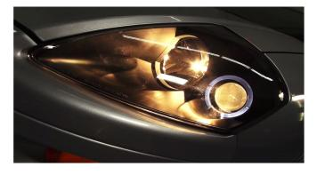
4) Lastly, test the new headlight assembly. Low beam and high beam will only come on individually and will not stay on together. Above is for reference only. Halo LED's require additional wiring; Please refer to our wiring guide at www.spyderauto.com
