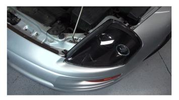
3) Once the assembly is removed and the harness is disconnected, attach the new Spyder harness to the OEM harness as shown in figure (2), remount the headlight, and reinsall the mounting bolts that were removed in figure (1).
