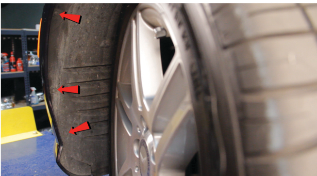
9) Remove [3x] plastic retainers securing the fender liner to the fascia.
