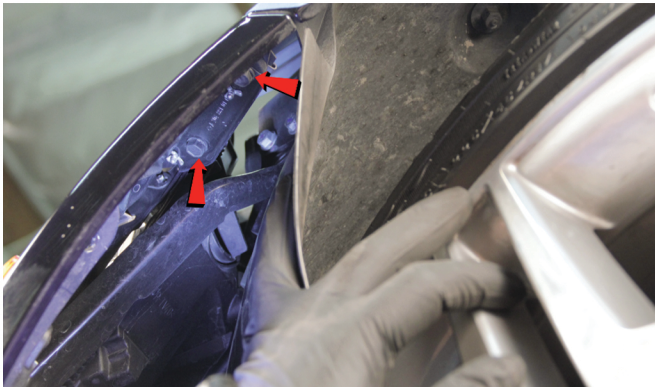
11) Remove [2x] 10mm bolts securing the fascia to the fender.
