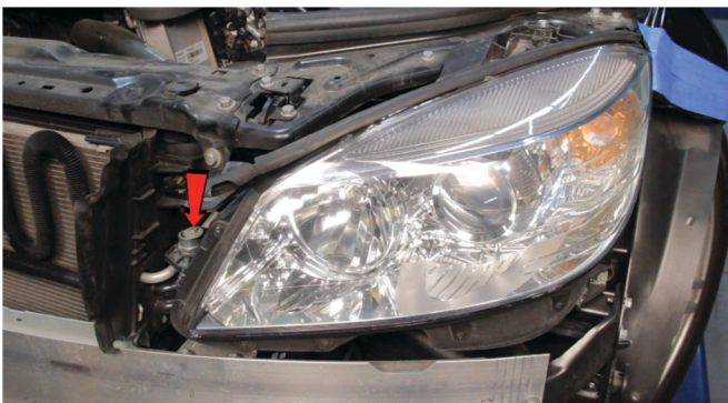
15) Remove [1x] 8mm bolt securing the headlight.
