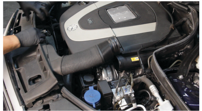
32) Seat the intake tube panel.
