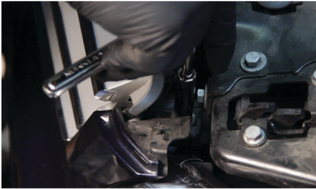
29) Reinstall [1x] 10mm bolt behind the grille to secure the fascia.
