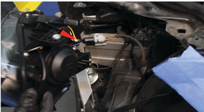
21) Reconnect the headlight harness to the Spyder headlight.
