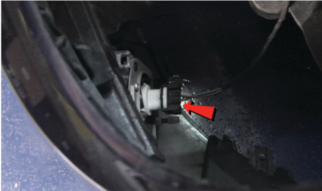
23) Reconnect the fog light wiring harness.
