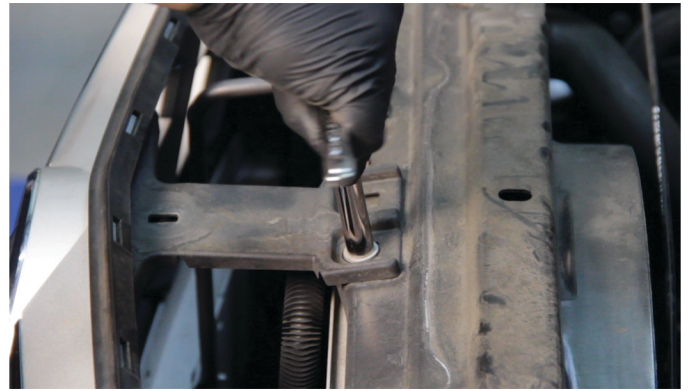
30) Reinstall [1x] 10mm grille bolt to secure the fascia.
