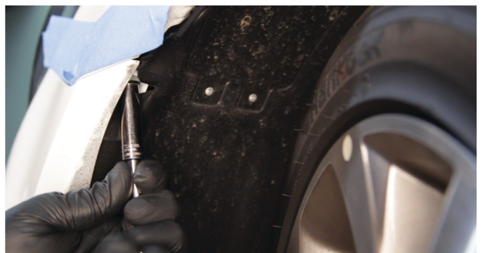
22) Reinstall the 10mm bolt that secures the corners of the fascia in the wheel well.
