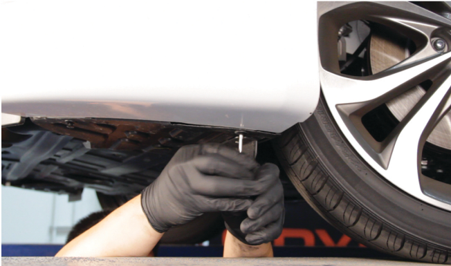
23) Reinstall [2x] Phillips Retainers that secure the fascia from below on each side.
