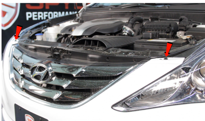
3) Remove [2x] 10mm bolts securing the corners of the fascia.
