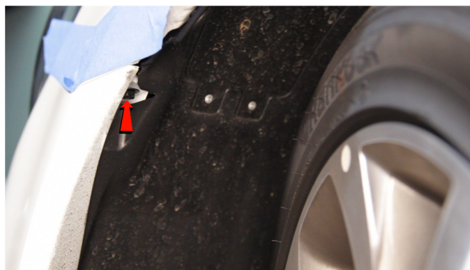
4) Remove the 10mm bolt securing the corner of the fascia in the wheel well.
