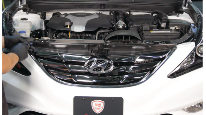
24) Reinstall [6x] Phillips Retainers that secure the fascia along the top edge of the grille.
