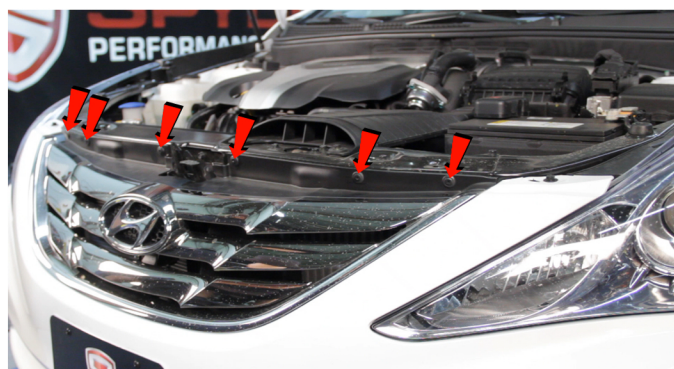
2) Remove [6x] Phillips Retainers securing the fascia.
