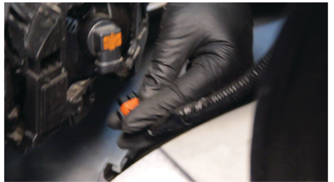
20) Reconnect the fog light wiring harness [if equipped].
