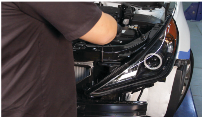
19) Reinstall [2x] 10mm bolts to secure the headlight. Note that the lower 10mm bolt is not used for the Spyder headlight.
