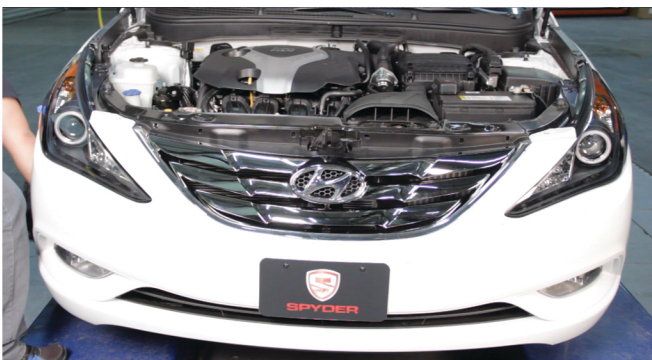
21) Seat the bumper fascia, being sure that the edges are properly seated.
