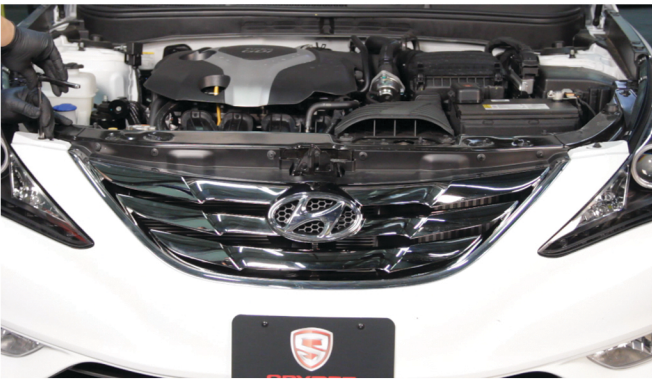
25) Reinstall [2x] 10mm bolts to secure the fascia.
