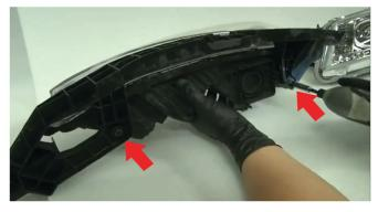
6) Next, once the head light has been removed you will notice it contains a bracket that helps seat the head light to the frame, this will need to be removed and installed on your Spyder head lights. Using the 10mm socket remove the (2) 10mm bolts, place the bracket on the new head light and secure it down with the (2) 10mm bolts previously removed.
