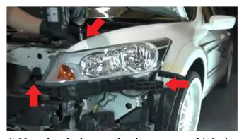
4) Now that the bumper has been removed it is time to unseat the head light. There are (3) 10mm type bolts that secure the head light down to the frame, locations are shown by arrows. Using the 10mm socket and ratchet, unscrew the (3) bolts from the head light and set them aside.
