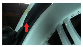
2) Next, there is (1) Phillip type screw that secures the bumper to the fender. Using the Phillips screw driver, remove that screw. This step will need to be done to both driver and passenger sides of the bumper.
