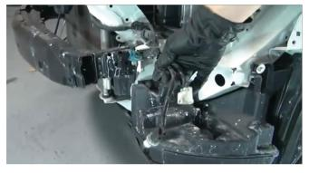
5) Before the head light can be taken off, all sockets must be unclipped from the back housing of the head light. You will need to leave the signal bulb attached to its socket on the harness, this will be placed later in your Spyder head light housing.
