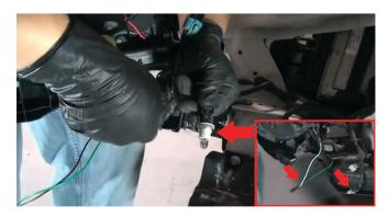
7) The next step is to connect the OEM harness to the new head light. Insert the signal bulb and sockets into their designated clips on the back of the head light. You will need to connect your corner parking light to the designated (Black, Green, White wires) socket, remove bulb to insert it. Be sure you are lining up the black ground wires on both sides when connecting.
