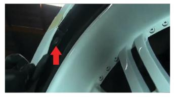
10) Next, move up to the fender lining, replace the Phillip type screw to secure the bumper to the fender.
