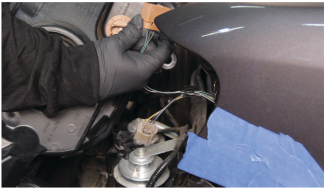
13) Disconnect the turn signal harness, then remove the headlight.
