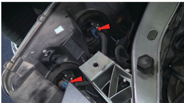
15) Disconnect the high beam and low beam harnesses, then remove the headlight and set it aside.
