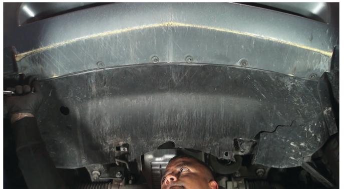
32) Reinstall [6x] 7mm bolts to secure the fascia to the undertray.
