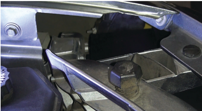
27) Reinstall [1x] 10mm nut & [1x] 10mm bolt hidden inside the fender to secure the fascia to the fender.
