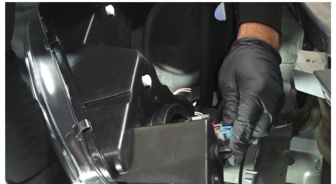
20) Reconnect the low beam harness.
