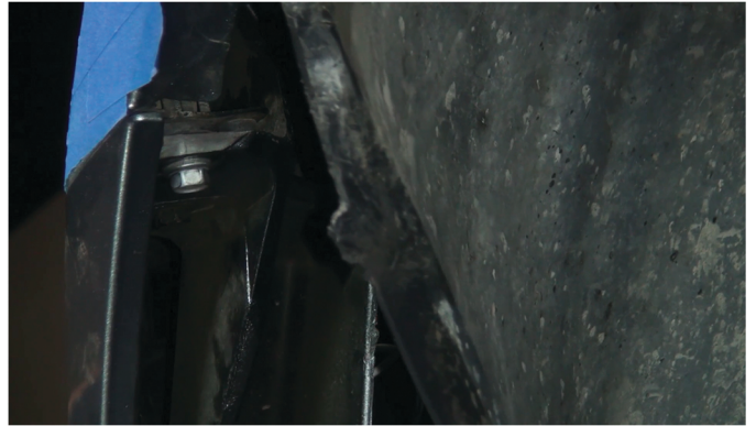
30) Reinstall [2x] 10mm bolts to secure the fascia to the fender.
