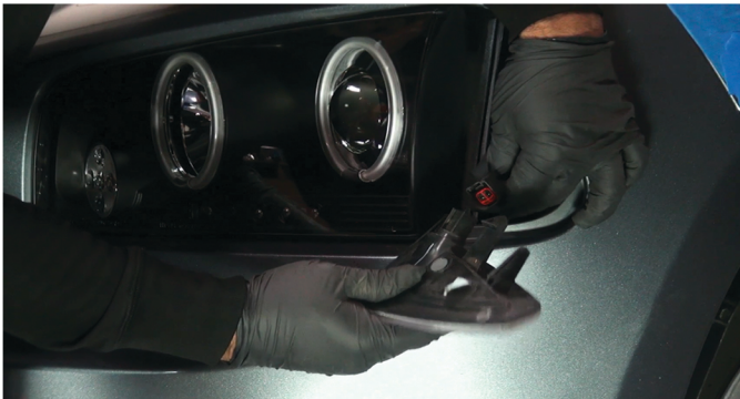
28) Reconnect the corner lamp harness.
