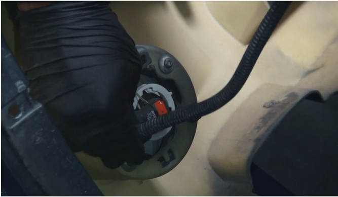
24) Reconnect the fog light wiring harness.
