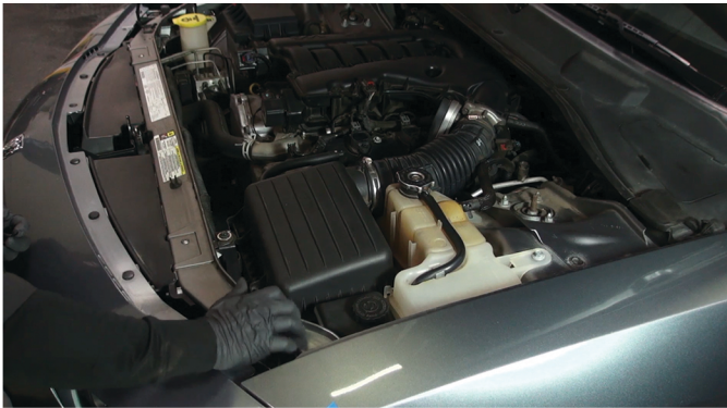
26) Reinstall [6x] plastic retainers along the header panel to secure the front fascia.
