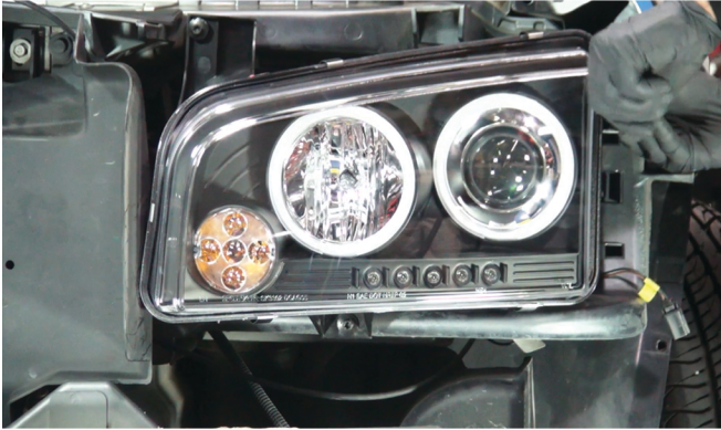
23) Reinstall [3x] T-30 Torx screws to secure the headlight.
