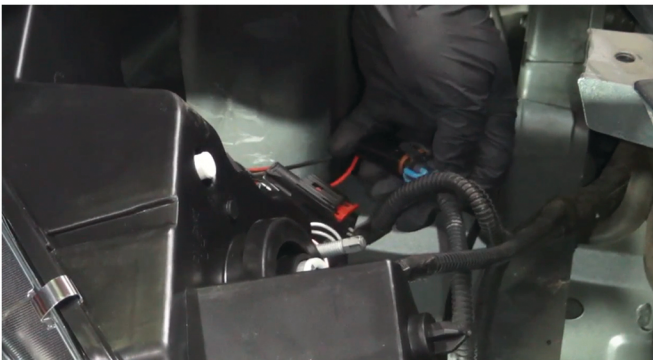
21) Reconnect the high beam harness.
