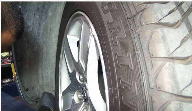
31) Reinstall [4x] plastic retainers to secure the fender liner.
