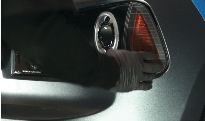
29) Seat the corner lamp by gently pushing the corner lamp back into place.
