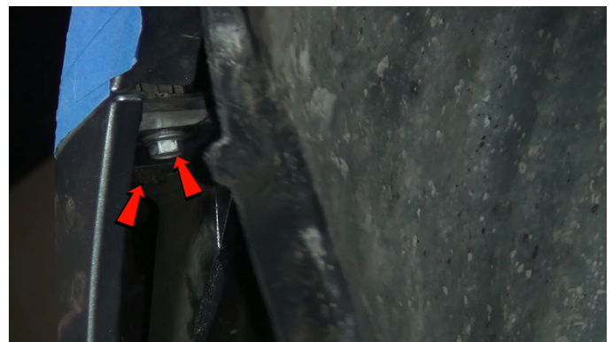
4) Remove [2x] 10mm bolts securing the fascia to the fender.
