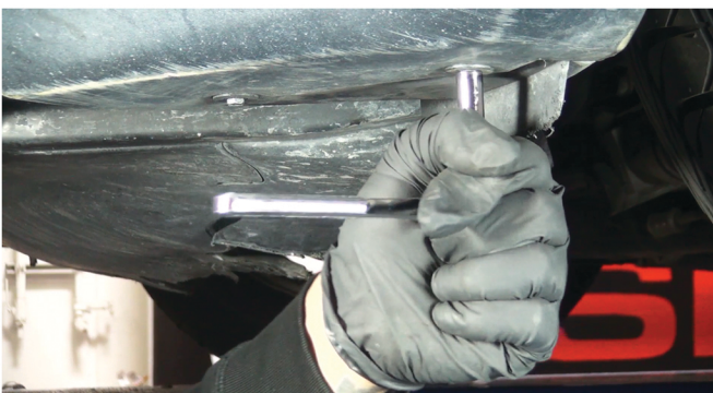
33) Reinstall [2x] 7mm bolts to secure the bottom corner of the fascia on each side.
