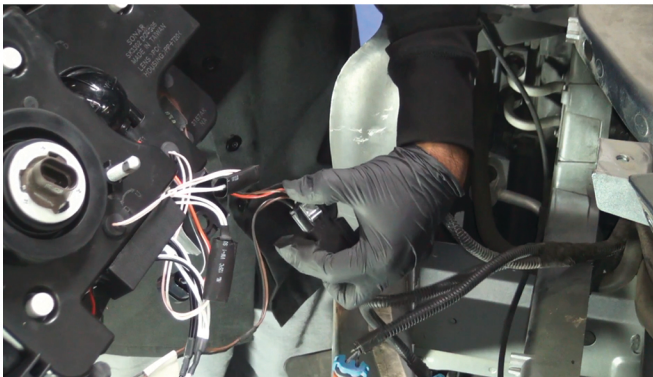
19) Reconnect the park/turn signal harness.
