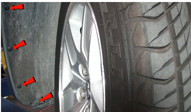
3) Remove [4x] plastic retainers securing the fender liner.
