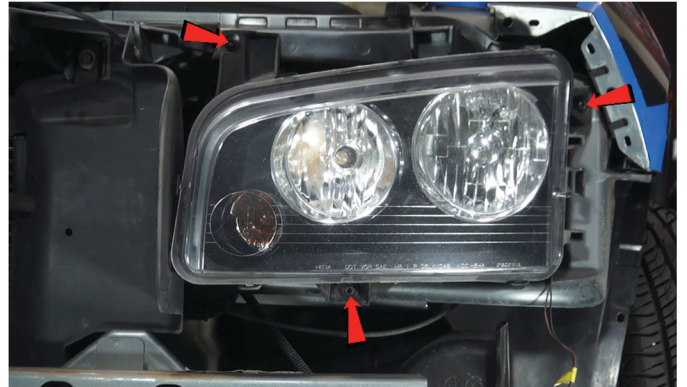
12) Remove [3x] T-30 Torx screws securing the headlight.
