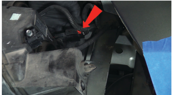
14) Disconnect the park/turn signal harness.
