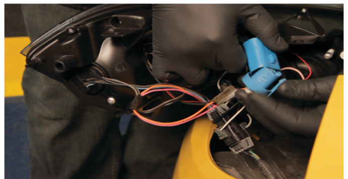
10) Reconnect the headlight wiring harness.
