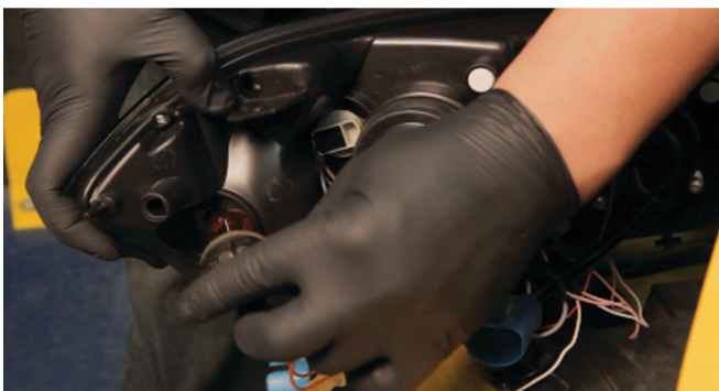
9) Reinstall the turn signal socket into the Spyder headlight.
