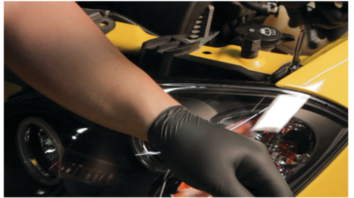
12) Reinstall [2x] 10mm bolts to secure the headlight.
