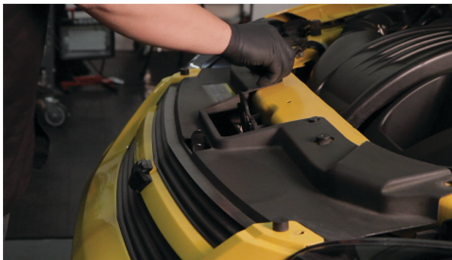
13) Reinstall [6x] plastic retainers to secure the fascia.
