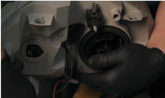
5) Remove the turn signal socket from the headlight.
