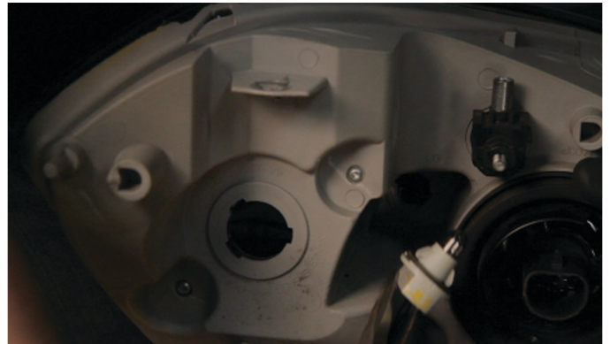
6) Remove the city light socket from the headlight.
