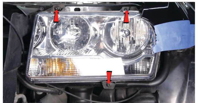
10) Remove [3x] 10mm (T-30) bolts securing the headlight.
