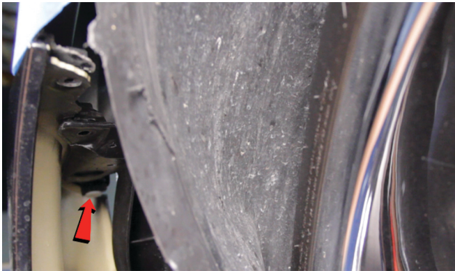
23) Reinstall [1x] plastic retainer to secure the fascia to the fender.
