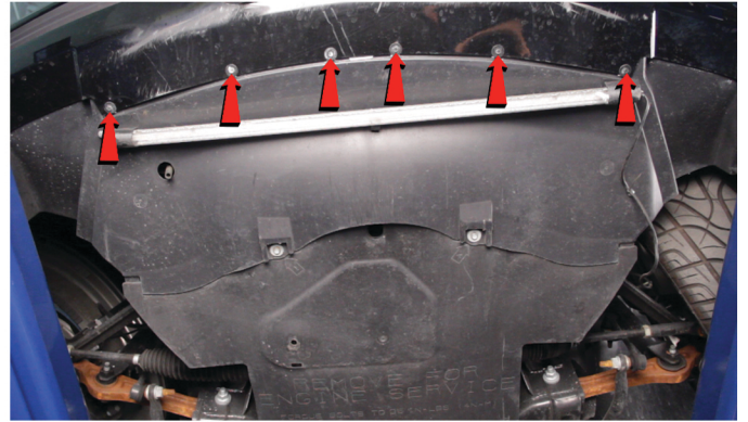
6) Remove [6x] 7mm bolts securing the fascia to the undertray.
