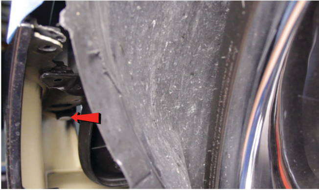
5) Remove [1x] plastic retainer that secures the fascia to the fender.
