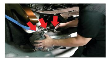
6) Next, you will need to remove the head light from the vehicle. Before it can be removed there are three sockets that are connected to the back of the head light. Twist these counter clockwise until they click.
