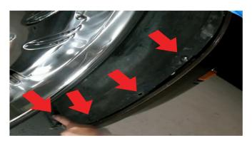
2) Next, detaching the fender liner from the bumper. Using the Pannel Popper pry the (4) plastic faseners from their mounting holes.
