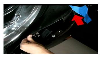
3) Next you will need to remove the 10mm bolt that is secured behind the fender liner. Use the 10mm socket or wrench to unscrew it from its bolt hole. Clips and bolts will need to be removed from both sides of the bumper.
