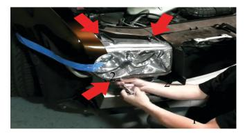
5) Now that the bumper has been removed locate the (3) 10mm bolts that secure the head light down. There will be two on the top and one below. Use the 10mm socket or wrench to unscrew them from there bolt holes.
