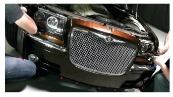
9) Place the bumper back by liining up the grill and corners with there mounting holes. You will need to replace the (4) clips on the grill, the 10 mm bolts on both bumper corners, (4) clips on both sides of the fender liners and (8) 8mm bolts on the bottom to secure the bumper back in place.
