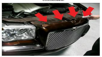
1) The bumper will need to be removeed to install your new Spyder head lights. First you will start by removing the top (4) clips from the grill area. Using the Pannel Popper pry the (4) clips from their mounting holes.
