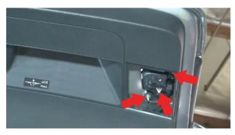
7) Once the access panel has been removed you will now be able to get to the two (2) 10mm bolts that need to be removed in order to unmount the tail light. Before completely removing from the lift gate, disconnect the harness (middle red arrow) so that the assembly can come free.
