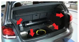
1) Open your trunk and locate U-Liner. Using the pannel popper tool, gently pry the liner free and set taside for later. The trunk liner covering will now be able to be pulled back.
