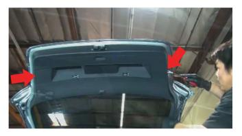
6) With the lift gate still open, using a flat head screw driver or pannel popper tool, gently pop each side of the lift gate open to reveal the second set of tail lights. Set the panels aside for later use. See figure 7 for bolt locations.
