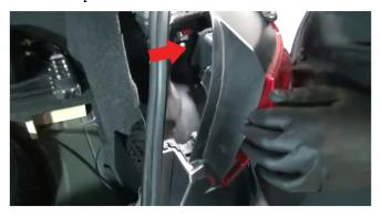
3) Next, gently pull outwards from the back of the tail light to get it free. Still attached will the be tail light harness (arrow). With moderate force, pull the harness apart from each other to unlatch it from the tail light.
