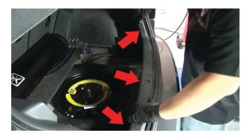
9) Once the panels have been replaced, get the U-Liner that was removed from earlier and place back into position. Make sure the trunk liner in placed under the U-Liner before snapping back into place. With a little pressure the U-Liner should pop back into its original location, and you're done!
