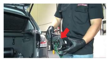
8) Now we will be reinstalling the tail light. Before remounting the tail light assembly, make sure that the gasket is in place before placing back onto the car. Place the new spyder tail light assembly back into mounting location and be sure to feed the wires through the opening. Reinstall the two 10mm bolts, then attach the harness, and replace the panel by pushing it back into position.
