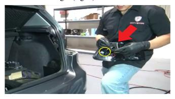
4) With the new Spyder LED tail light, make sure you place the square gasket over the wiring harness before reinstalling the tail light. This will prevent condensation issues. Once this has been done, you can now reseat the tail light. (fig, 5)
