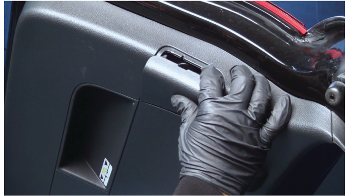
12) Remove the inner tail light access cover.
