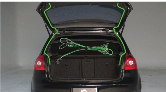
9) Route the green and black outer to inner tail harness included with your tail light through the body along the path marked here. The green and black outer-to-inner harness MUST be connected for inner LEDs to light up.
