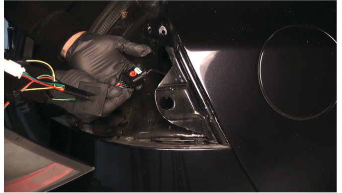
6) Connect the Spyder outer tail light to the outer tail light wiring harness.
