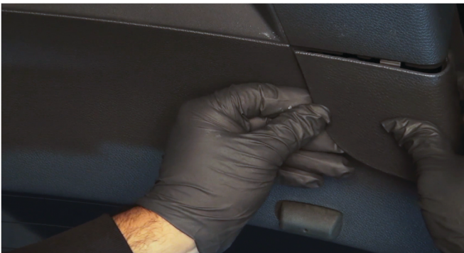
21) Close the inner tail light access panel.
