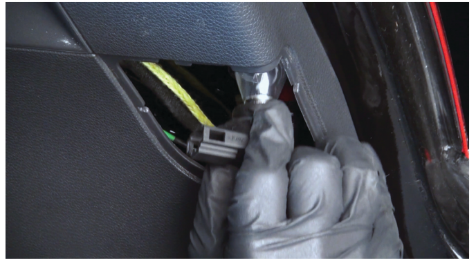
14) Remove the reverse bulb socket for access. Never touch exposed bulbs with bare hands.
