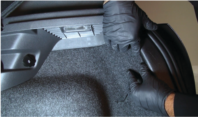
11) Tuck the harnesses away, then close the access flap.
