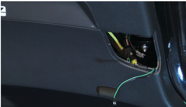
19) Reinstall [2x] 10mm nuts to secure the inner tail light.
