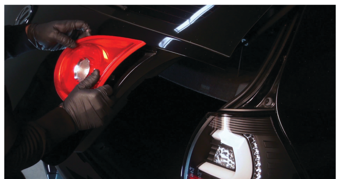
16) Unseat and remove the inner tail light.
