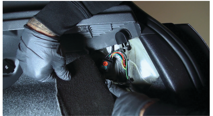
8) Reinstall [2x] 10mm nuts to secure the outer tail light to the body.
