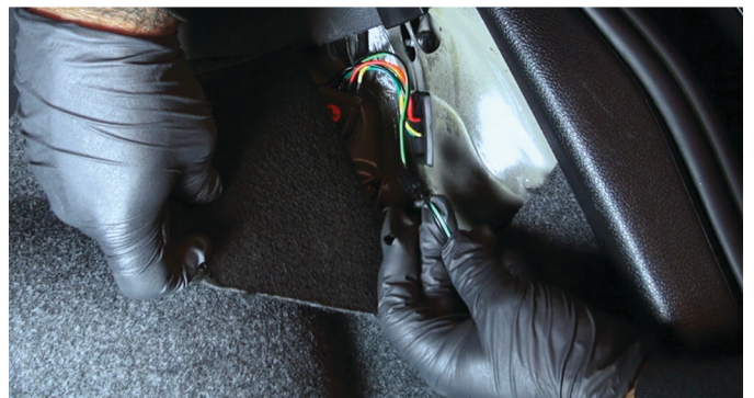
10) Connect the green and black outer-to-inner tail harness to the main outer tail light harness.
