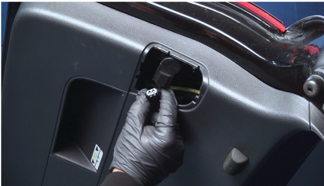
13) Disconnect the inner tail light wiring harness.
