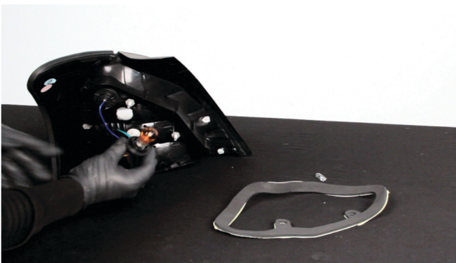
7) Install the included amber bulb into the yellow and black wire turn signal socket. Reinstall the socket.
