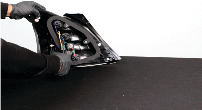
9) Install the included adhesive gasket onto the backside of the tail light.
