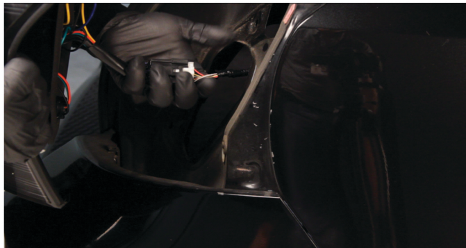
10) Connect the tail light harness.
