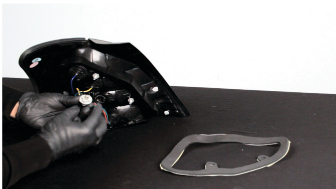
8) Install the included small 194 bulb into the green and black wire socket. Reinstall the socket.
