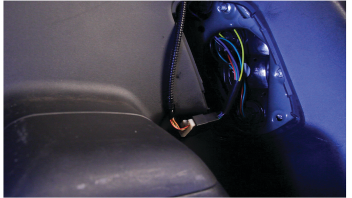
12) Reinstall [2x] 10mm nuts to secure the tail light.
