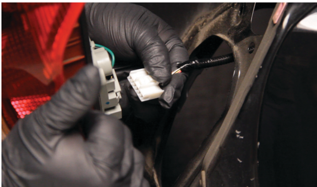
5) Disconnect the tail light harness.
