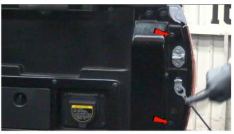
2) Remove the [2x] 10mm bolts securing the tail light.
