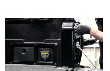
9) Reinstall the two 10mm bolts securing the tail light.
