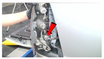
4) Disconnect the wiring harness.
