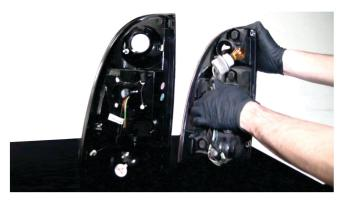
5) Remove the turn signal, brake/park lamp and reverse lamp sockets from your OEM tail light, then transfer the bulb socket harness to your Spyder tail ight. Never touch exposed bulbs with bare hands.
