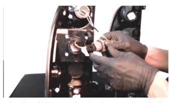
6) Reinstall the turn signal and reverse lamp bulb sockets into your Spyder tail light. Remove the brake lamp bulb from the socket, and install the Spyder socket insert. Align the black wire side of the socket with the black wire side of the insert.
