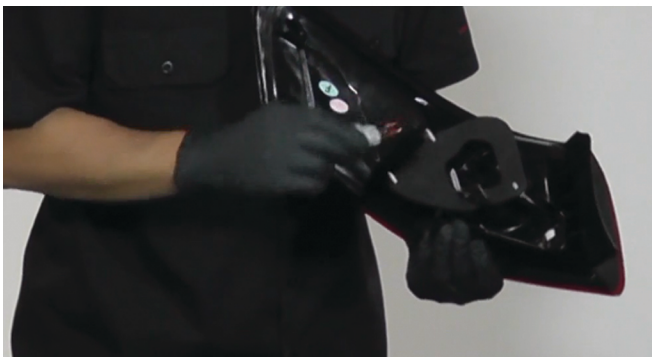
27) Transfer the turn signal socket to the Spyder outer tail light.
