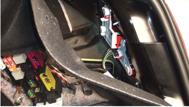
5) Disconnect the tail light wiring harness.
