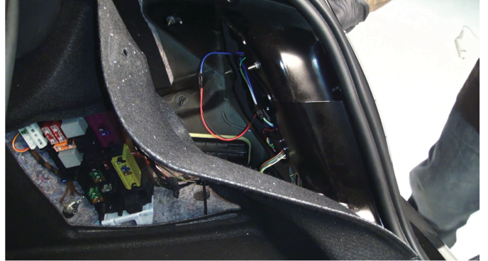
12) Reinstall [4x] 8mm bolts to mount the tail light.
