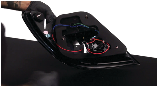
9) Be sure the gasket is properly mounted. Your Spyder tail light is now ready to install.
