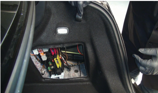
13) Replace the trunk liner, then reinstall the grocery hook and its retaining stake.
