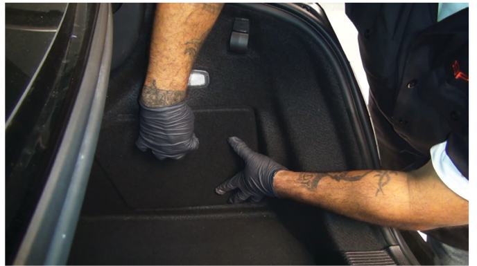
14) Reinstall the access panel, then lock the panel.
