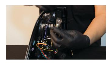
8) Install the bulb into the Spyder reverse lamp socket, then reinstall the socket securely into the Spyder tail light housing, then you're ready to install the Spyder LED tail light.
