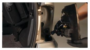
9) Connect the Spyder tail light to the tail light wiring harness.
