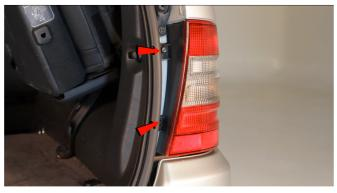
2) Remove the [2x]10mm/Flathead bolts securing the tail light.
