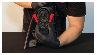
5) Remove the bulb panel from the OEM tail light by squeezing the retainer tabs together to release it.
