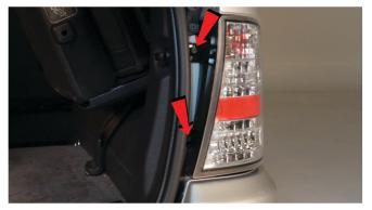
11) Reinstall [2x] 10mm/flathead bolts securing the tail light.
