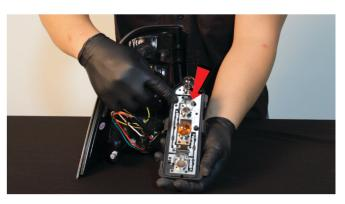
6) Remove the reverse lamp bulb from the 2nd position on the bulb panel. Never touch exposed bulbs with bare hands.
