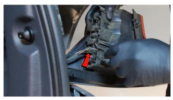
4) Disconnect the wiring harness.
