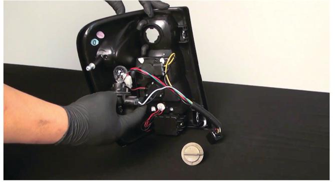
6) Transfer the reverse lamp bulb to the white and black wire reverse lamp socket of the Spyder tail light. Reinstall the socket, then your Spyder tail light is ready to install.
