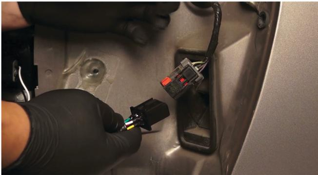
7) Connect the Spyder tail light harness to the main wiring harness. Then push down on the red tab to lock the harness.
