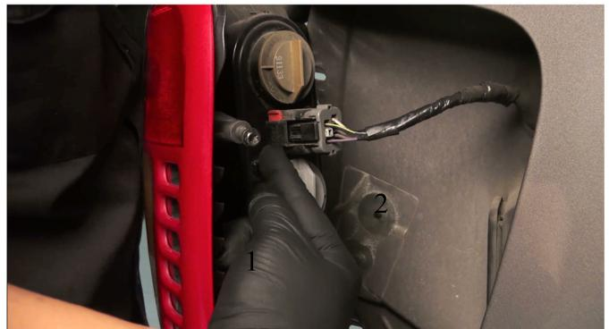
4) Disconnect the tail light wiring harness. Push up on the red tab to unlock the harness, disconnect the harness and remove the OEM tail light.
