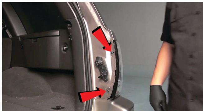
9) Transfer the turn signal bulb to the yellow and black wire bulb socket. Transfer the reverse lamp bulb to the white and black wire bulb socket. Then reinstall the sockets. Now your Spyder tail light is ready to install.
