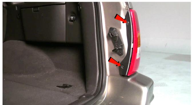
2) Open the tail light access panel by releasing the two tabs.
