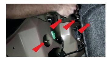
7) Use the four included 8mm nuts to secure the SPYDER tail light to the body.
