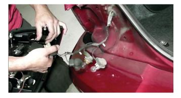
5) Locate the SPYDER LED tail light. Disconnect each of the brake light bulbs and connect each of the three the socket insert harnesses. Line up the black wire side of the socket with the black wire side of the insert. If you do not do this, you can blow fuses and void your warranty. Leave the reverse bulb in place.
