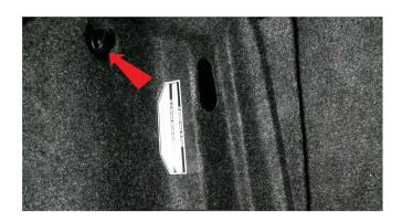
8) Replace the trunk liner and reinstall the plastic thumbscrew that secures the liner.
