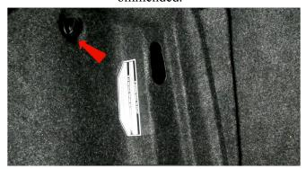
1) Open the trunk. Remove the thumbscrew securing the trunk liner.
