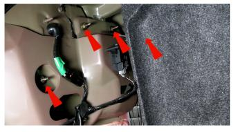
2) Peel back the trunkliner. Remove the four 10mm nuts securing the taillight (one is hidden by the trunk liner). Discard the 10mm nuts.
