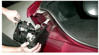
4) Remove the taillight bulbs from the sockets in the OEM tail light. Set aside the OEM tail light. You may wish to thread the 10mm nuts onto the studs of the OEM tail light, should you keep the OEMs.
