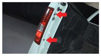
1) Open your tailgate and locate the (2)10mm bolts. Using the 10mm socket wrench/ratchet to remove the bolts and set them aside for later.
