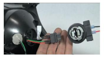
3) Once the turn signal bulb has been removed, you can now connect the Spyder harness. Make sure the Positive (red/green) and Negative (black) is properly connected or they will not work. Once this has been done, reinstall the reverse light bulb into the new housing.
