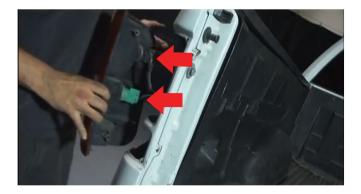
2) Next, gently pull outwards from the side of the tail light to remove freely. Still attached will be the tail light harness (arrow). Remove both bulb sockets by twisting counter-clockwise. Retain the reverse light bulb and only remove the turn signal bulb from the socket.
