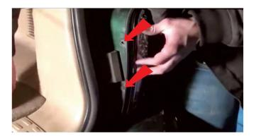
8) Reinstall the two phillips screws that secure the tail light, then close the tailgate/trunk.
