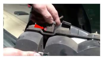
3) Remove the tail light harness by sliding the red retainer tab free, then disconnecting the harness. Then set the OEM tail light aside.
