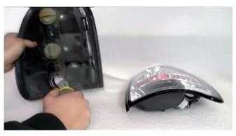
4) Remove the reverse lamp bulb from your OEM tail light by first removing the socket, then removing the bulb from the socket.
