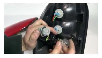
5) Transfer the reverse lamp bulb to the SPYDER tail light, installing the bulb fully into the reverse bulb socket, then reinstall the socket into the SPYDER taillight housing.
