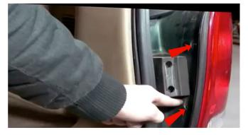
1) Open the tailgate. Remove the two phillips head screws securing the tail light.
