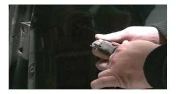
6) Before we can seat the tail light we must reconnect the harness. Locate the wiring harness connector on the SPYDER LED tail light and plug it into the OEM wiring harness socket, then slide the red tab to lock the harnesses together.
