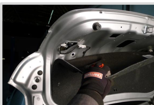
41. Pull trunk liner down
