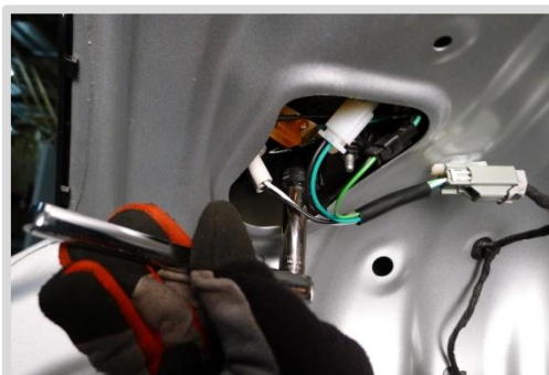
53. Tighten 2 10mm nuts
