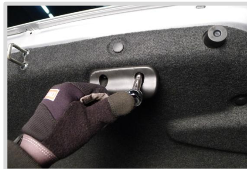
36. Remove 2 7mm bolts then the plastic handle
