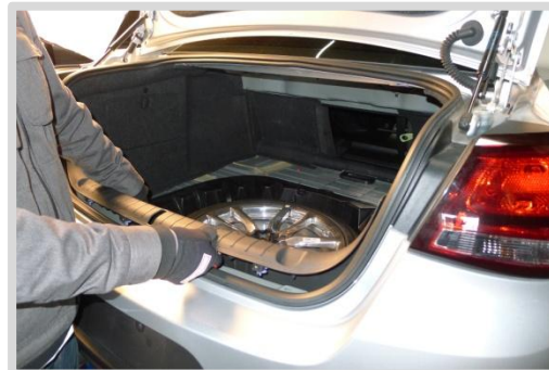
9. Remove rear trunk moulding
