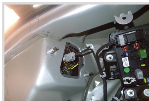
24. Pull trunk liner aside
