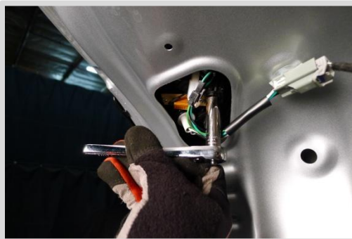
52. Tighten 2 10mm nuts
