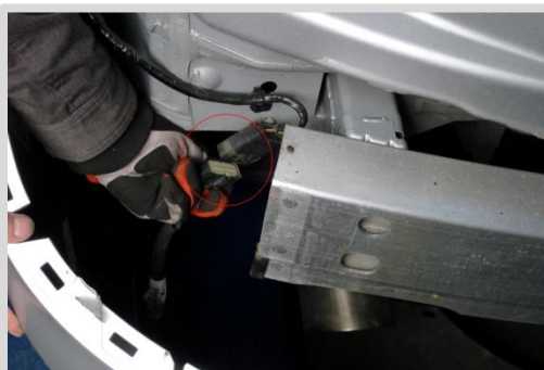
22. Disconnect backup sensor harness
