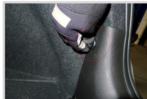
6. Remove 4 wing screws
