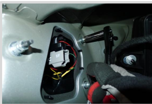
34. Tighten 3 10mm nuts
