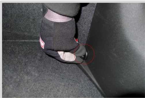
7. Remove 4 wing screws
