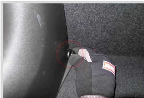
5. Remove 4 wing screws
