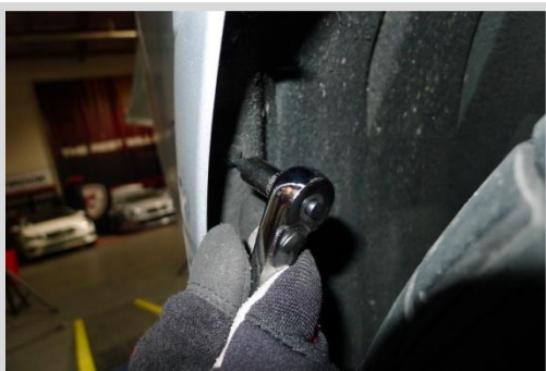
64. Tighten 5 T15 screws
