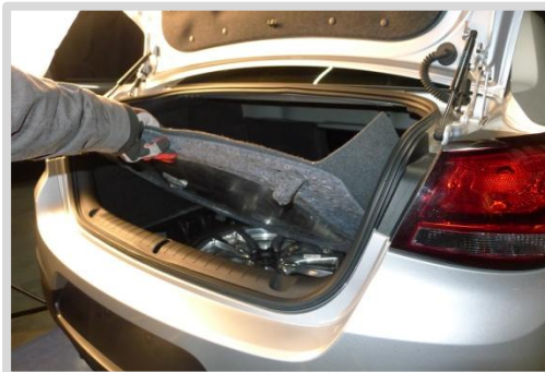
8. Remove trunk floor
