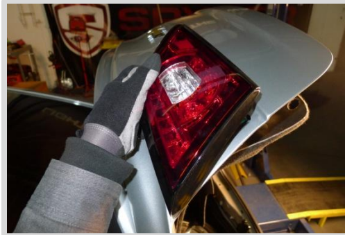
50. Position LED taillight onto trunk lid
