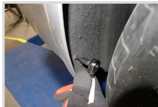
12. Remove 5 T15 screws
