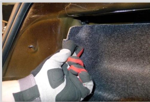
28. Replace 3 wing nuts and trunk liner
