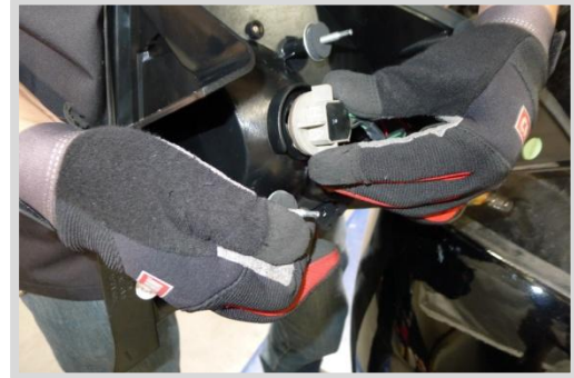
21. Install brake light socket
