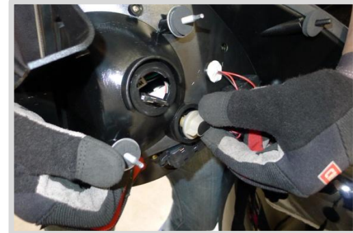
24. Install parking light socket
