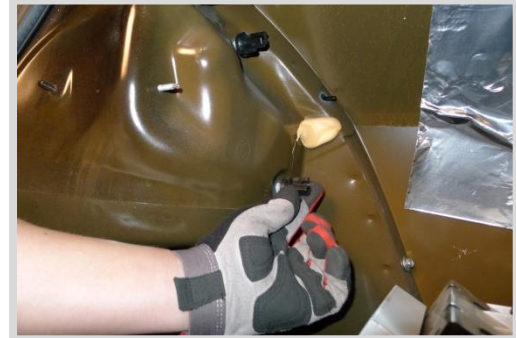
27. Replace 3 wing nuts and trunk liner
