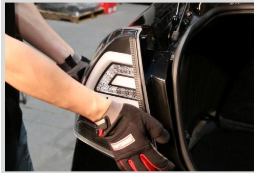
26. Place LED tail light on the car
