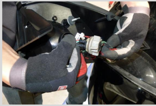
22. Connect LED connector to parking light socket.
