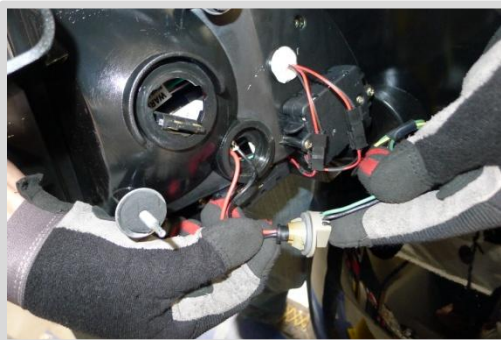
22. Connect LED connector to parking light socket.
