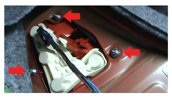
2) Once the panel has been removed, locate the (3) 8mm bolts securing the tail light. Remove these and the tail light harness from the bulb bracket.
