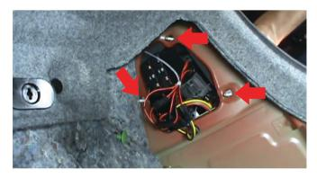
5) Next, seat the tail light onto the frame lining up the three bolt threads with their mount holes. Replace the (3) 8mm bolts. Once these are secure you can connect the wiring harnesses together.
