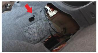
1) Open your trunk and locate the access panel covering the tail lights. Twist the knob to unlock the panel and remove it.
