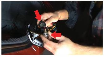
4) Taking the new Spyder outer tail light housing, remove the lower two sockets and insert the (2) bulbs removed from the old tail light. Place them in the sockets and replace the sockets back into the tail light housing. Be sure to seat the sockets flush and properly to prevent any moisture in the tail light.
