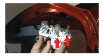
7) The next step is similar to the corner tail light installation. Remove the bulbs indicated by the arrows shown. You will need to insert these in to the designated sockets on the new Spyder trunk tail light.
