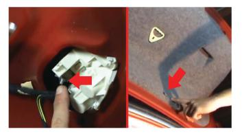
6) Now that the corner lights are complete you will need to install the trunk lights. Before you can get to the back housing of the trunk tail light you will need to remove several plastic fasteners that secure the trunk liner. Next, locate the 8mm nut that secures the light, unscrew this to remove.
