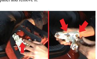
3) Next, remove the tail light and locate the tab on the bulb bracket, pinch the tab to remove it from the tail light. Next you will need to remove (2) bulbs from the bulb bracket. Bulbs that will need to be removed are indicated by the arrows shown.
