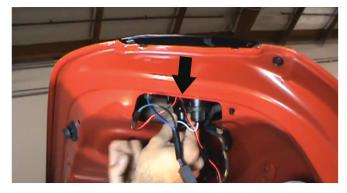
9) Next, seat the light on the trunk lining up the corners. To secure the light to the trunk you will need to install the bracket to hold the light onto the trunk then tie it down with the 8mm nut. Tighten the bolt down with the 8mm socket. The final step is to mount the resistor ballast. Peel off the red 3m plastic film and mount the resistor on a flush area. Note: be sure before mounting the resistor that the area is cleaned very well or it will not stick.
