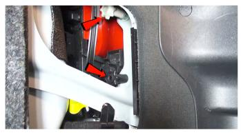
2) Remove [2x] plastic thumbscrews securing the outer tail light.
