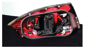
5) Remove [2x] Phillips screws securing the bulb plate to the tail light. Remove the side marker socket from the OEM tail light.
