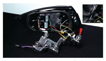
6) Remove the bulb plate, then transfer the reverse lamp from the bulb plate to the black and white wire reverse socket of your Spyder tail light. Then reinstall the socket. Never touch exposed bulbs with bare hands. Your Spyder tail light is now ready to install.
