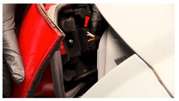
4) Disconnect the tail light wiring harness.
