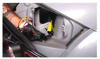
7) Connect the Spyder tail light to the wiring harness.
