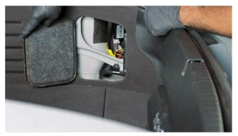
1) Open the trunk and open the tail light access panel.
