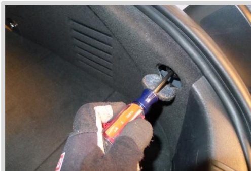
5. Loosen taillight mounting screw
