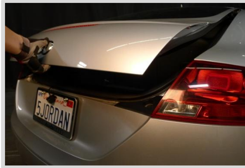
5. Loosen taillight mounting screw
