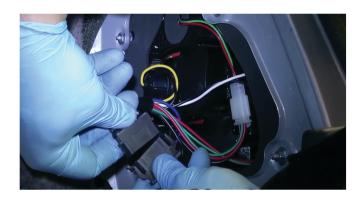
9) Reconnect the wiring harness, then replace the trunk liner and reinstall the two plastic retainers.
