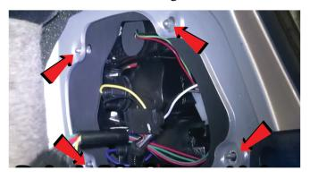
8) Reinstall the four 8mm nuts that secure the tail light to the body.
