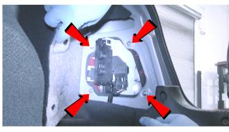
2) Remove the four 8mm nuts securing the tail light.
