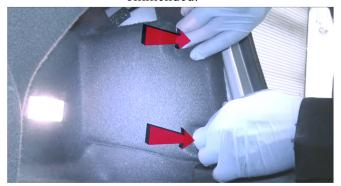
1) Open the trunk. Remove the plastic trunk retainers, then peel back the trunk liner to access the backside of the tail light.
