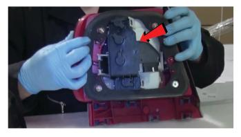
5) Remove the bulb mount bar from the OEM A4/S4 tail light. Release the mounting tabs to remove the bulb mount bar.
