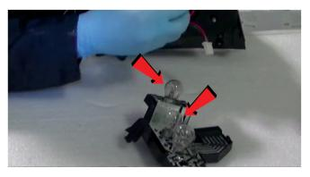
6) Remove the bulb from the raised position on the bulb mount bar and install it into the socket with black and white wires on the SPYDER tail light. Remove the center bulb from the bulb mount bar and install it in the socket with blue and black wires on the SPYDER tail light.
