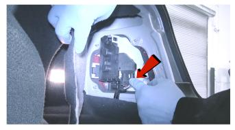
3) Disconnect the wiring harness plug. To disconnect the plug, push the side of the plug, then pry it outwards.
