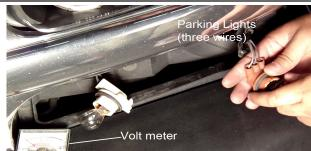
The volt meter has a positive (red) and negative (black) needles. First turn on the parking light and signal on. Then Pinch the Negative needle to a ground or negative wire(as shown). Then Pinch the Positive wire to one of the color wires on the turn signal.
