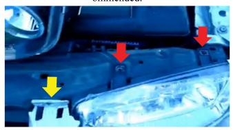
1) Begin by opening your hood and locating the (1) Hex bolt and (2) 8mm bolts. These will need to be removed before the head light can be ejected. Using your Torx bit and 8mm socket, remove them from their mount holes.
