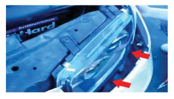
7) The next step is to replace the (2) Hex bolts on the bottom of the head light. Using the Torx bit, tighten these bolts back into place.
