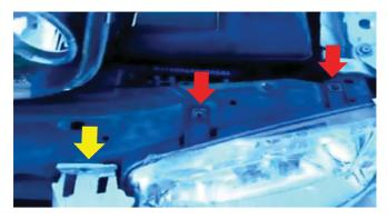
9) Lastly, replace the (1) Hex bolt and (2) 8mm bolts on top. Using your Torx bit and 8mm socket, tighten them into their mount holes.
