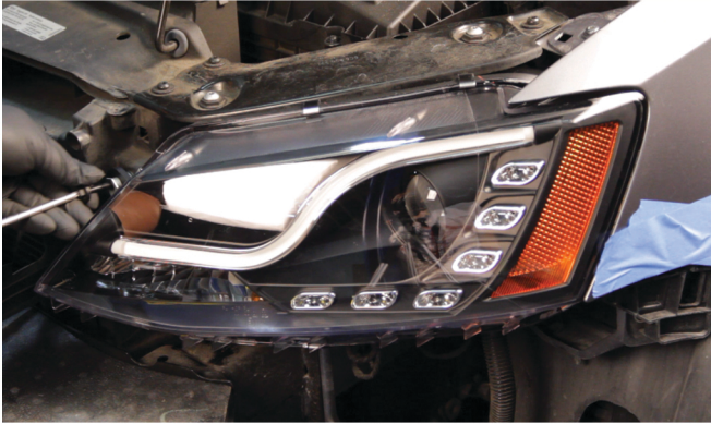
17) Reinstall [3x] T-30 Torx screws to secure the headlight.
