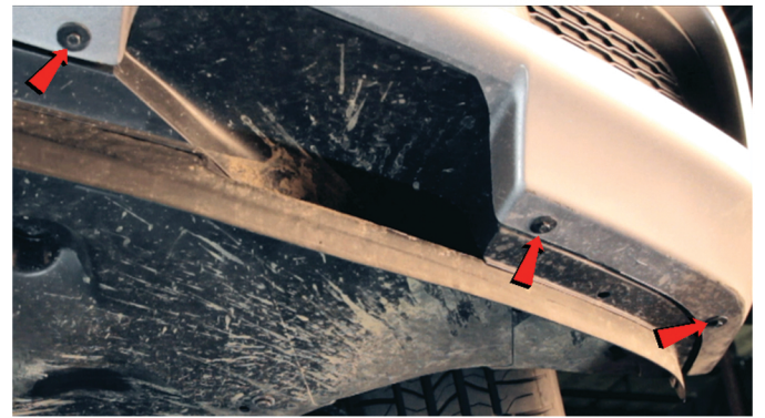
8) Unseat the front bumper fascia by pulling it up to unseat the fascia retainer hooks, then pull the edges out and ease the fascia back.
