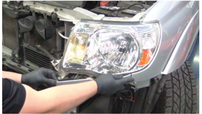
12) Remove the headlight garnish by gently swinging it outwards and away.
