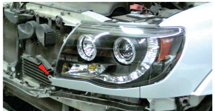
28) Reinstall [1x] plastic retainer to secure the garnish.
