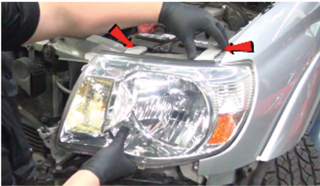
13) Release the headlight retainer tabs.
