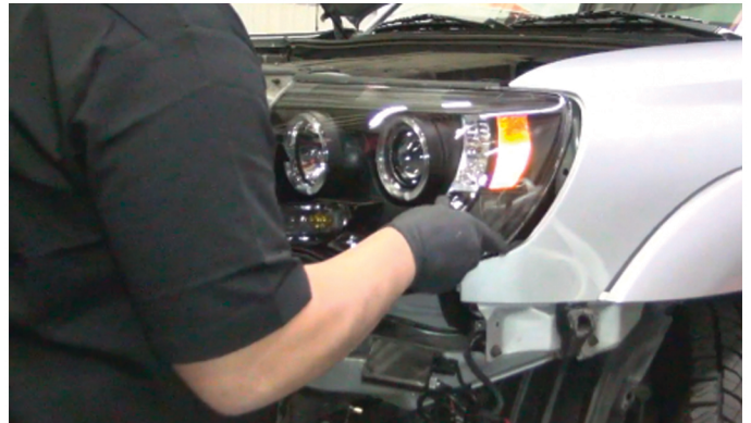
24) Seat the Spyder headlight, being sure to properly seat the headlight retainer tabs.
