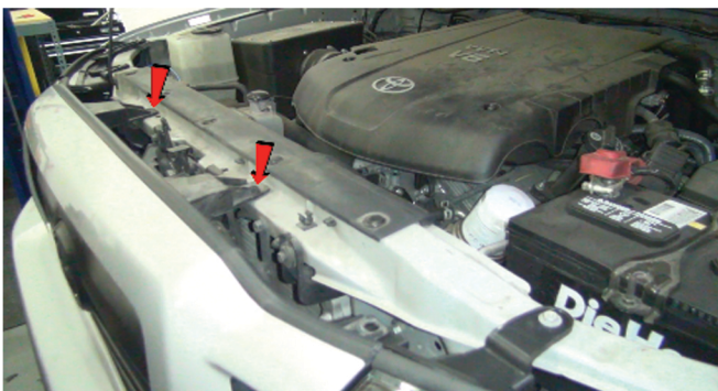
33) Reinstall [2x] phillips screws to secure the grille.
