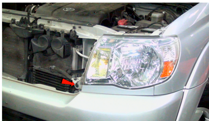
4) Remove [1x] plastic retainer securing the headlight garnish.
