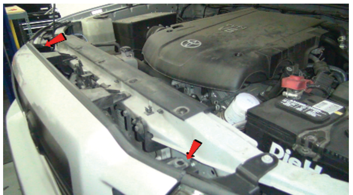
32) Reinstall [2x] plastic retainers to secure the grille.
