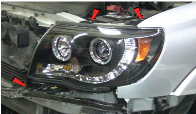
25) Reinstall [3x] phillips screws to secure the headlight.
