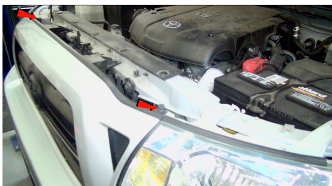
1) Open the hood, remove [2x] plastic retainers on either side of the grille.
