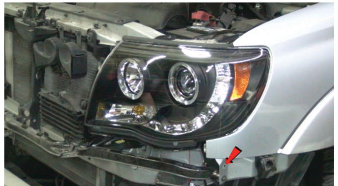
26) Reinstall [1x] 10mm bolt to secure the headlight.
