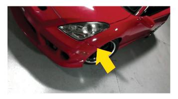
7) Now that the head light is secure, replace the front bumper and bolt it down. Begin by replacing the 10mm bolt that secures the bumper to the fender.
