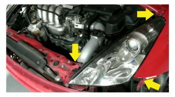
4) Now it's time to remove the head light. Begin by unbolting the (3) 10mm bolts that secure it down to the frame. Once those are removed, unseat the head light and begin to unhook the head light harnesses.
