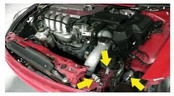
5) Once the head light is removed you will need to install the harnesses removed from your old head lights into your new Spyder head lights. Test your head lights before beginning reinstall process.
