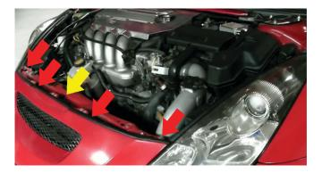
8) Replace the (4) 10mm bolts and (1) plastic fastener that secures the bumper to the frame. Be sure these are secures properly
