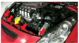
1) Begin by opening your hood and locating the (4) 10mm bolts and (1) plastic fastener that secures the bumper to the frame. Using the 10mm socket remove them from their mounting holes.
