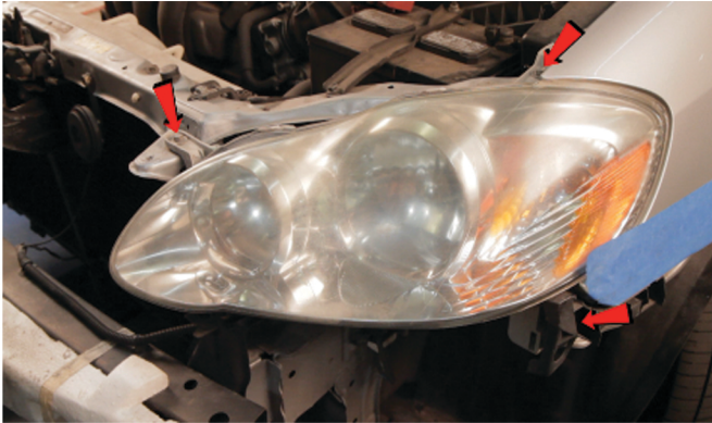
5) Remove [3x] 10mm bolts securing the headlight.
