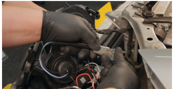
16) Connect the low beam harness.
