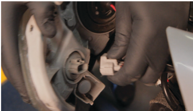
7) Disconnect the turn signal harness.
