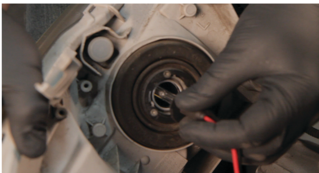
9) Disconnect the low beam harness.
