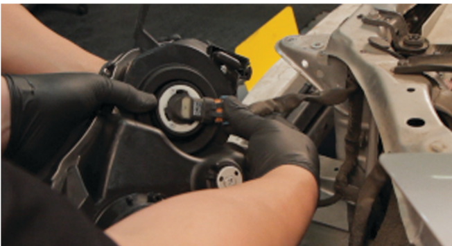
15) Reconnect the high beam harness.
