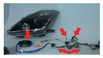
12) Here you will notice all parts removed from the original head light. From left to right: HID ballast, mount screws, HID bulb, igniter pack and wiring harness.
