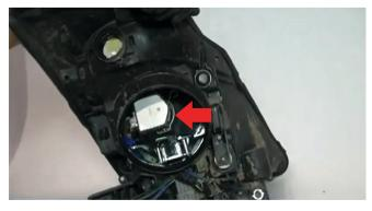
11) Next, the HID bulb and igniter pack will need to removed from the head light. Begin by removing the igniter pack off of the HID bulb. Next, unclip the HID bulb and remove it. Be sure your fingers do not come into contact with the bulb as this can cause the bulb to blow out when reinstalled.
