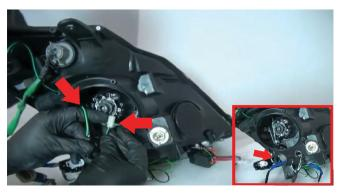
13) It is now time to install all items removed from your old head light onto your new one. Begin by inserting the turn signal bulb into its socket then inserting the HID bulb into the projector socket, secure it down with its clip. Next, feed the wiring harness into the head light through the inlet below the projector housing. Connect the green wiring with black clip from the head light with the green wire with white clip from the harness.
