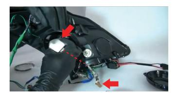
14) Next, secure the igniter box onto the back of the HID bulb and feed the igniter harness through the projector housing and out through the bottom where the ballast will mount. Replace the cover to the projector housing and using the removed screws, screw it back down into place.
