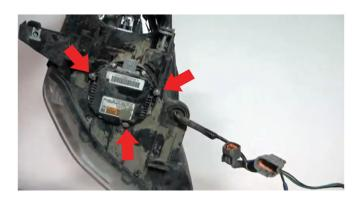
8) Turn the head light over and locate the ballast. Using your Phillips screw driver, unscrew the (3) Phillip type screws to remove it.
