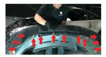
21) Lastly, replace the (12) 10mm bolts to the bottom of the bumper to secure it back to the splash guard and frame and you are done.
