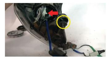
10) Start pulling out the wiring harness until you have reached (2) white sockets clipped together. Remove the sockets from one another to enable the full release of the wiring harness. Next, unseat the rubber seal attached to the head light and pull the entire harness free, seal is shown circled above.
