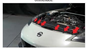
1) Begin by opening your hood and locating the (6) plastic fasteners that secure the bumper to the frame. Using the panel popper, pry the fasteners free. Set them aside for later use.
