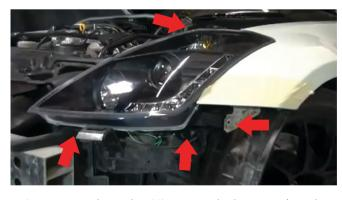
18) Next, replace the (4) 10mm bolts securing the head light to the frame. Place the bumper support foam back onto the vehicles support brace as removed.
