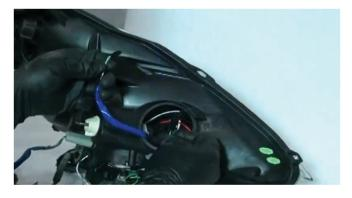
16) Next you will need to open the high beam housing by removing the rubber capping. There will be a small connection wire inside, taking the blue wrapped wiring from the harness previously inserted into the head light, connect the two together and then replace the rubber seal.
