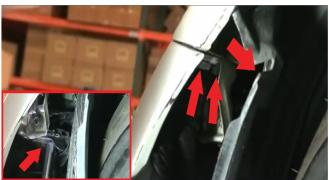
2) Next, you will need to remove (3) 10mm bolts from the fender well, pull back the fender liner to locate them. (1) bolt will be offset from the two and can be seen a bit further back as shown.
