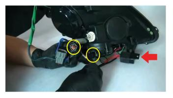
17) Once everything has been closed up and secured begin to connect the rest of the wiring harness. From the relay there will be (2) socket both with red and black wring, connect these to their designated socket on the harness. Connect the corner light connector to the white and back clip from the head light.
