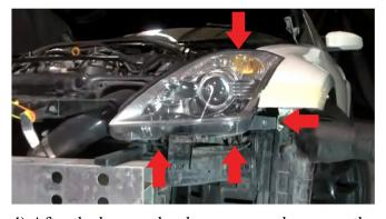
4) After the bumper has been removed, remove the bumper support foam. Removing the foam will expose (1) of (4) 10mm bolts that will need to be removed to unseat the head light. Location of the bolts are shown above.
