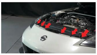
19) Seat the bumper back onto the vehicle and replace the (6) plastic fasteners on top to secure the bumper back to the frame.
