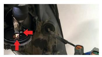
9) Once you have unseated the ballast, you will need to unscrew (1) Phillip type screw then disconnect the igniter pack harness. The clip may be a little hard to pinch, use the tip of the panel popper to assist in removing the clip.
