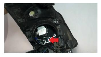
7) In order to reach the harness from inside the head light, unscrew the projector housing cover off. Next, unclip the harness beside the igniter pack as shown.
