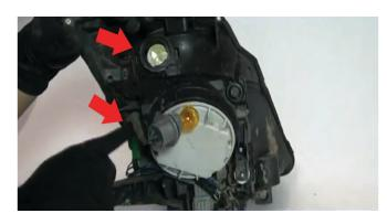
6) Next, you will need to transfer several components to your new Spyder head lights. Begin by removing the complete wiring harness. Unseat all bulbs and sockets top to bottom.
