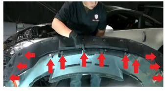
3) To fully remove the bumper you will need to unscrew (12) 10mm bolts that secure the bottom of the bumper to the frame and splash guard. Once they have been removed, unseat the entire bumper from the vehicle.
