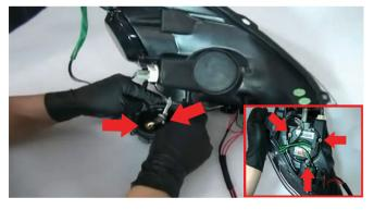
15) The next step is to connect the igniter harness into the ballast by inserting its clip into the socket. Replace the screw into the igniter harness bracket to secure the harness down to the ballast. Position the ballast onto its mounting points and replace the (3) screws that secure the ballast to the head light.
