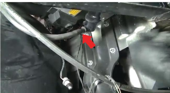
9) Below the head light you will need to remove the water hose from the washer mechanism. You will remove the washer mechanism later, for now only remove the hose. Note; there will be water in the lines so be sure you are ready to catch that bit of water.
