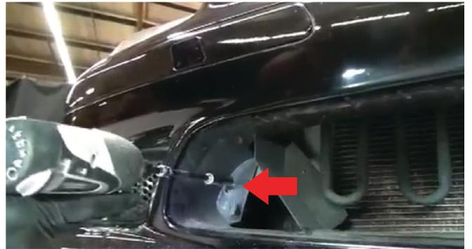
20) Below you will need to install the (2) 10mm bolts that hold the center of the bumper to the frame. Once these are on you can replace the grill. Simply line up the tabs and gently push them into place.
