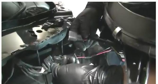
16) The next step is to connect the OEM harnesses to the new head light harnesses. Match them up correctly and give them a slight tug to insure they are snapped in. Once this is done reseal the head light back in place.
