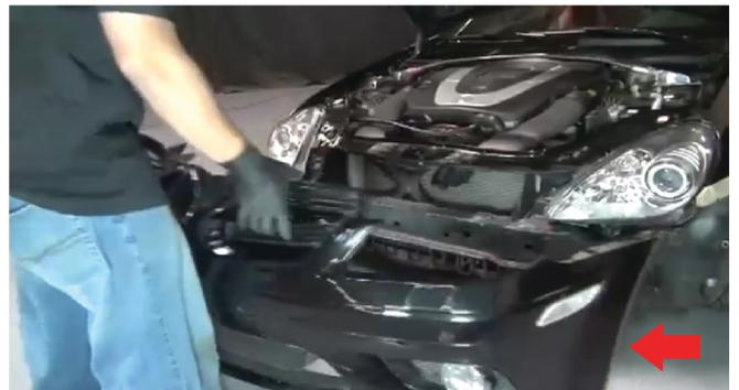
8) Now the bumper is removable from the vehicle but to fully detach it you will need to remove the fog light sockets and corner light sockets. Simply twist the light sockets from the housings. Note: there is a temperature sensor on the driver side that will need to be removed as well.
