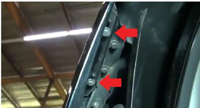
3) Next, gently peel back the fender liner to expose the (2) 10mm bolts that secure the bumper to the fender. Use your socket wrench to remove these.
