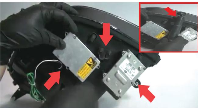
15) Next, replace the (2) ballasts and nozzle clip down first. Once you have screwed these all back into place first then replace the washer nozzle onto the clip and last screw to hold it into place.
