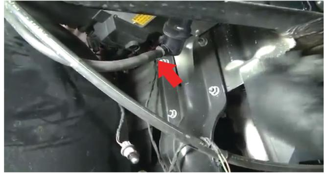
18) Replace the water hose back to the washer nozzle. Be sure to secure it tightly to that it does not come loose when used.
