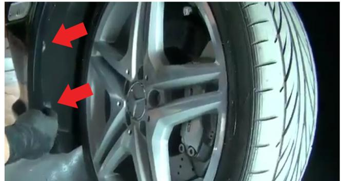
2) Now locate the (2) 10mm bolts you will need to remove on the fender liner. Use your socket to unbolt these two to access the bumper from behind.
