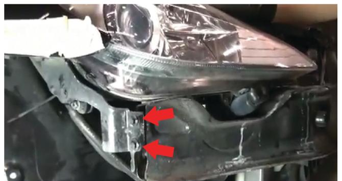
10) Now, unbolt the (2) 10mm bolts from the corner of the head light to release it from the frame. Be sure when removing the head lights that you have removed all bolts shown on both sides. Unplug all head light wiring leading to the head lights from their connectors.
