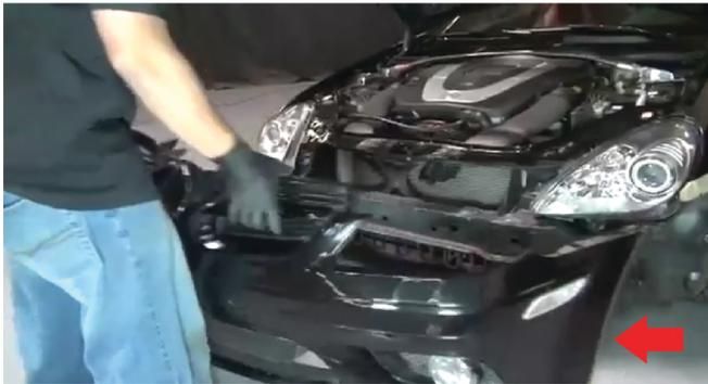
19) Next, replace the all fog light harnesses and temperature sensor on the driver side. Mount the bumper, carefully lining up the mount holes with the bolts holes. It will be easier to secure the center two bolts on the grill to that you can properly secure the corners and lower grill.
