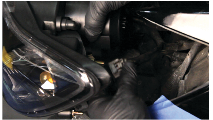
42) Reconnect the turn signal harnesses.
