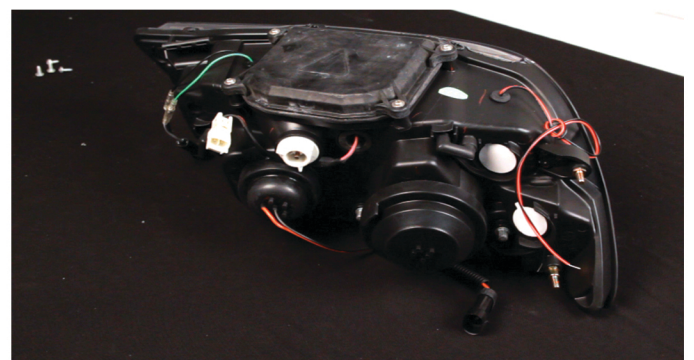
34) Seat the ballast cover and reinstall [4x] phillips screws to secure the cover.
