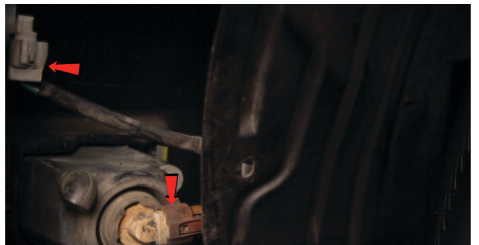
46) Reconnect the sidemarker and fog light harnesses.
