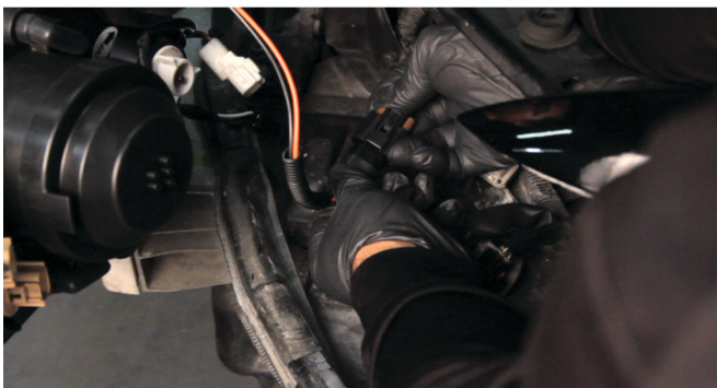
39) Reconnect the high beam harness.
