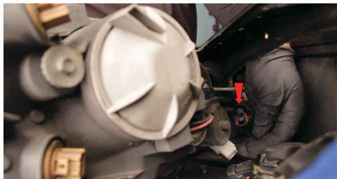
16) Disconnect the high beam harness.
