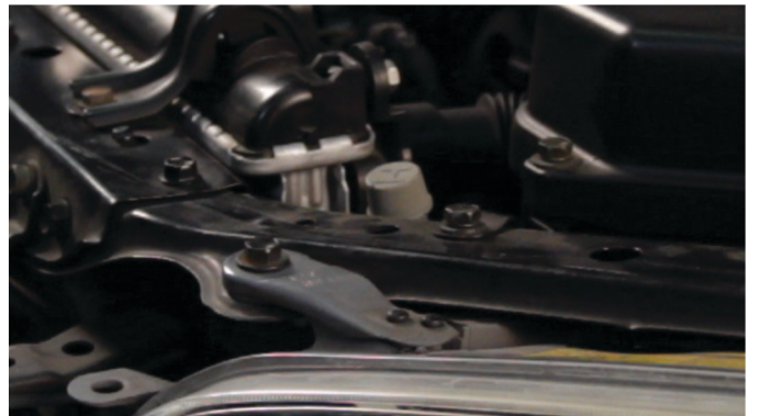
44) Reinstall [1x] 10mm bolt to secure the headlight.
