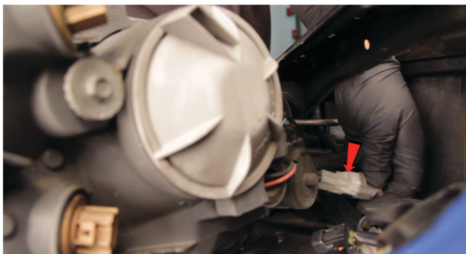
15) Disconnect the HID input harness.
