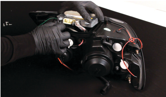
31) Seat the ballast and reconnect the HID input harness.
