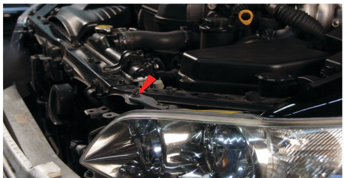
10) Remove [1x] 10mm bolt securing the headlight.
