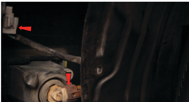
9) Disconnect the sidemarker and fog light harnesses.
