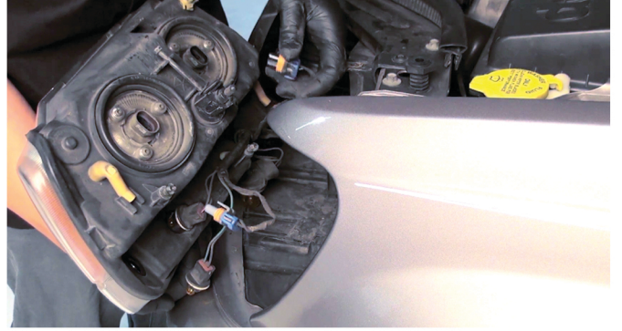
6) Disconnect the high beam harness.
