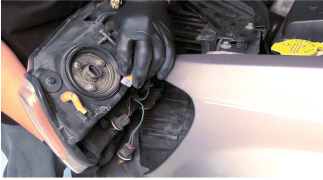
5) Disconnect the low beam harness.
