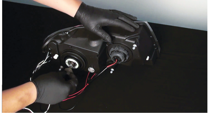
8) Install the low beam bulb into the Spyder headlight. Be sure to check the bulb gasket and replace it if worn. Your Spyder headlight is now ready to install.
