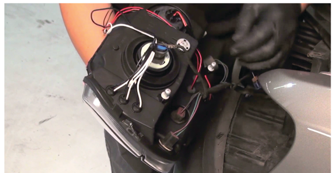
10) Reconnect the low beam harness.
