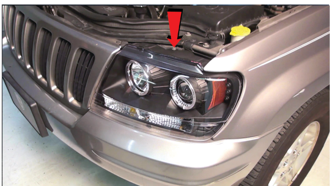
13) Reinstall the 7mm headlight retainer bolt.
