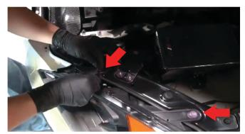
6) Once the headlight has been reseated, reinstall the two 10mm bolts that will lock the new light in place. Repeat this entire process for the other side. Then reattach the grille, and all 8 phillips screws to secure it into place.
