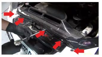
1) Open your hood and locate the 8 phillips screws that you will need to remove in order to get the grille off. You will need to do this in order to be able to fully remove the headlight.
