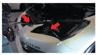
5) Now to reinstall the headlight. Locate your OEM harness you removed, and connect it with the new spyder harness. The connector should "click" in place when attached correctly.
