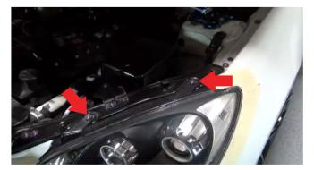
2) Once the grille has been removed, locate the two 10mm bolts shown here and unscrew them. Once these have been removed, set the screws aside as you will reuse them later.
