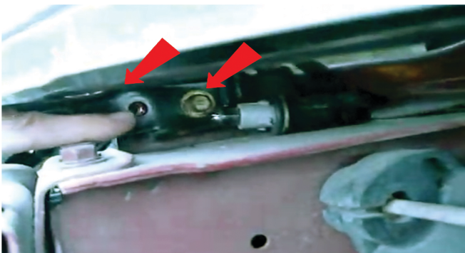
15) Reinstall the two 10mm bolts securing the headlight from below.
