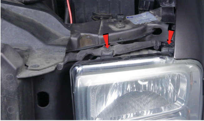
5) Remove [2x] 5.5mm bolts securing the headlight.
