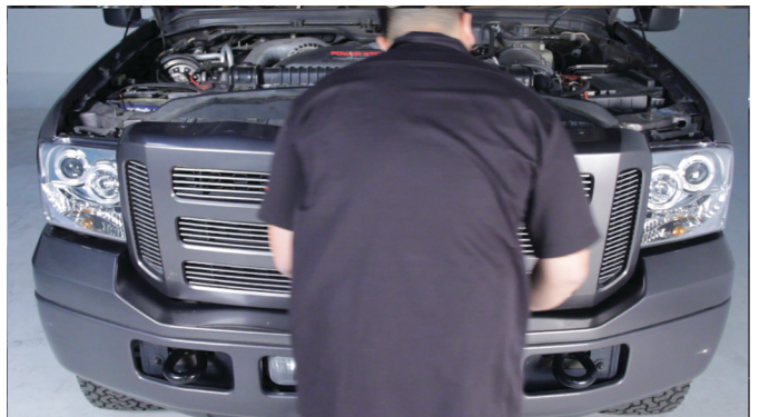
20) Seat the grille, being sure it fits properly into its mounting tabs.
