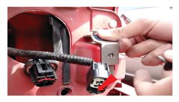
7) Locate the special bracket included with your SPYDER headlight. Install the bracket as shown in the location where the corner lamp bracket used to mount.
