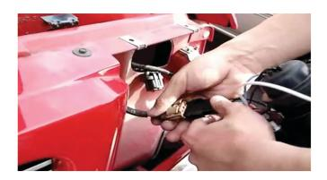
9) Connect the SPYDER headlight harness to the factory wiring harness.
