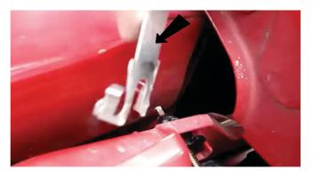
11) Locate the special retainer tab included with your SPYDER headlight. Install the special retainer tab in place of the old outer retainer tab that we removed.
