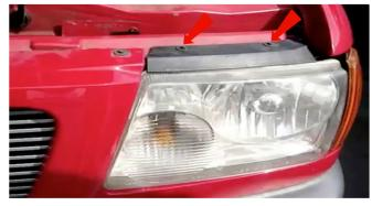
1) Remove two 5.5mm Bolts Securing Headlight Trim Cover.
