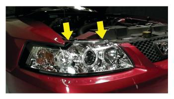
6) Replace the (2) metal fasteners to secure the head light to the frame of the vehicle and you are done.
