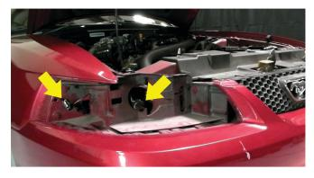
5) Next, remove the Low/High beam clip from the bulb with socket, connect that clip into the Spyder head light harness. Insert and secure the corner parking light into the corner housing of the head light, seat the head light on the vehicle
