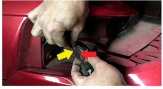
4) After the power wires have been connected, twist the (2) Black halo ground wires together from the Spyder head light. Again taking the parking light socket from the vehicle, locate the Black wire on the outer left of the socket. Splice the Black ground wires to the Black harness wire using a Splice connector.
