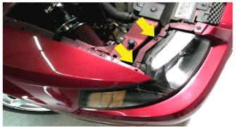
1) Begin by opening your hood and locating the (2) metal fasteners that secure the head light to the frame. Remove them by pulling up and out, this will release the head light.
