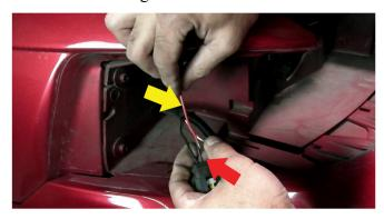
3) Next, the halos will need to be connected. Twist the (2) red halo power wires together from the Spyder head light. Next, Taking the parking light socket from the vehicle, locate the Brown wire in the center of the socket. You will need to splice the Red power wires to the brown wire using a Splice connector.
