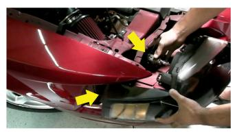
2) Once the metal fasteners are removed the head light can be slid out. Remove the Low/High beam and corner light sockets from the back housing of the head light indicated by the arrows.
