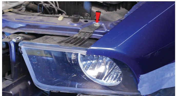
14) Support the headlight as you remove the final [1x] 10mm bolt securing the headlight to avoid dropping the headlight.
