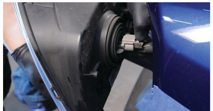
16) Disconnect the headlight wiring harness, then remove the headlight and set it aside.
