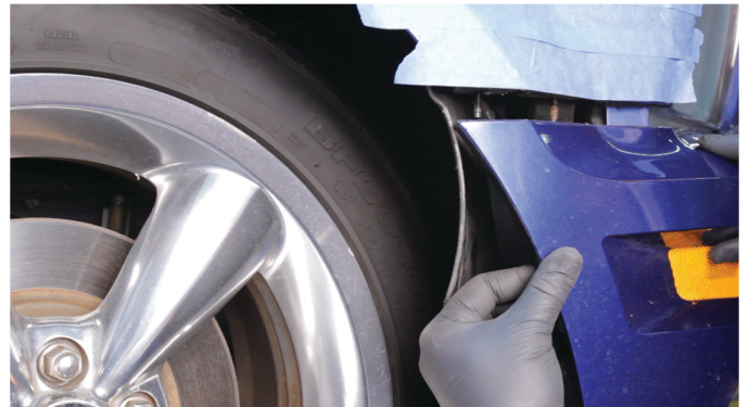
8) Pull down on the corner of the fascia to unseat it from the fender stud.
