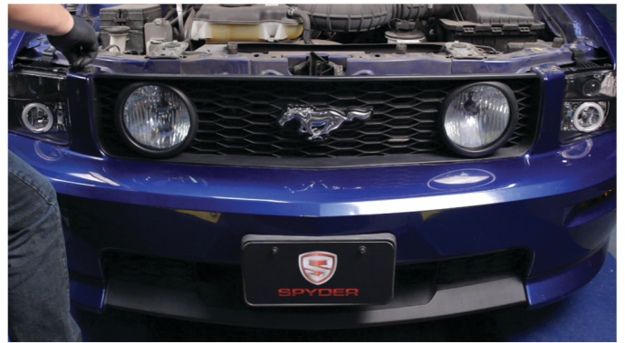
26) Reinstall [2x] 10mm bolts to secure the fascia on either side of the grille.
