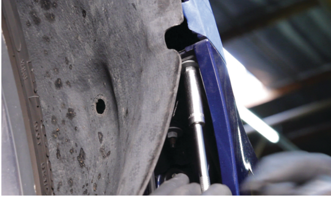
29) Reinstall [2x] 10mm nuts to secure the fascia to the fender.
