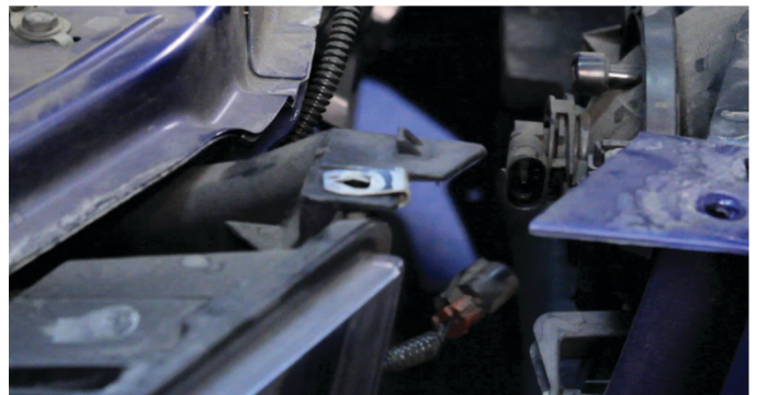
10) Disconnect the turn signal socket.
