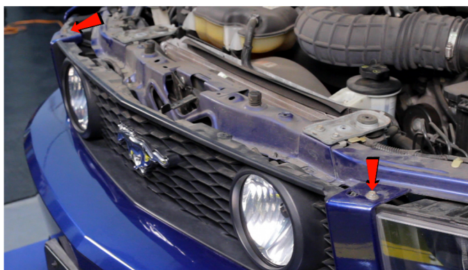
4) Remove [2x] 10mm bolts securing the fascia on either side of the grille.
