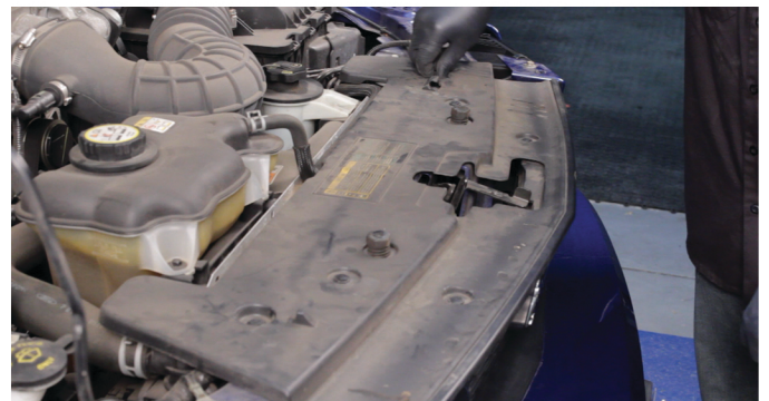
28) Reinstall [6x] plastic retainers to secure the filler panel.
