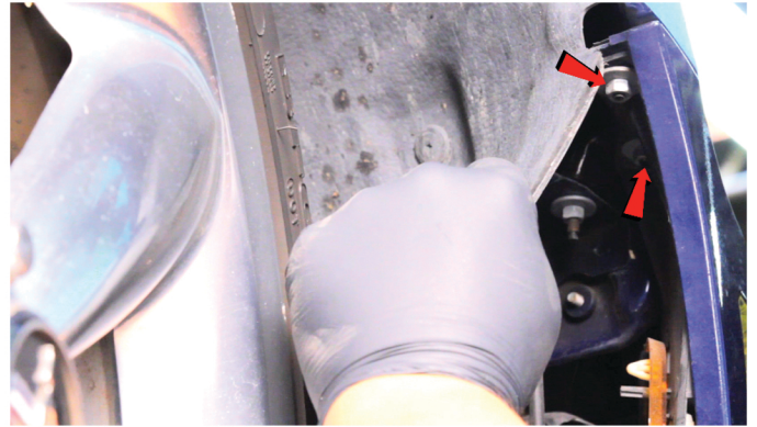
6) Remove [2x] 10mm bolts securing the fascia to the fender.
