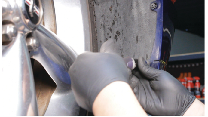
30) Reinstall [3x] phillips screws to secure the fender liner.
