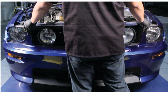
9) Release the mounting tabs on either side of the grille, then you can unseat the fascia.
