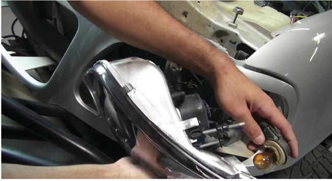
5) Locate your SPYDER headlight. Install the headlight bulb/socket and the turn signal bulb/socket.
