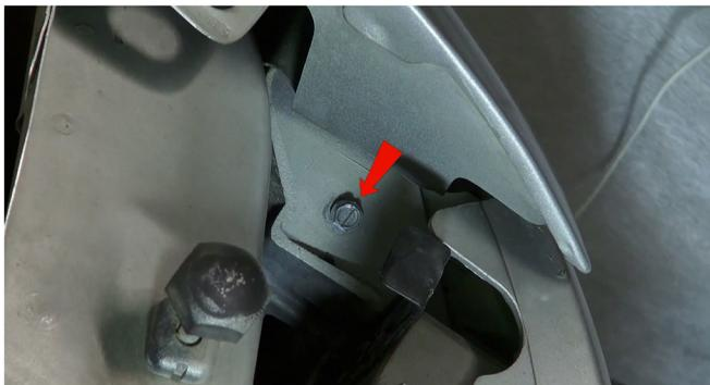
1) Open the hood. Remove the flathead screw securing the corner lamp.
