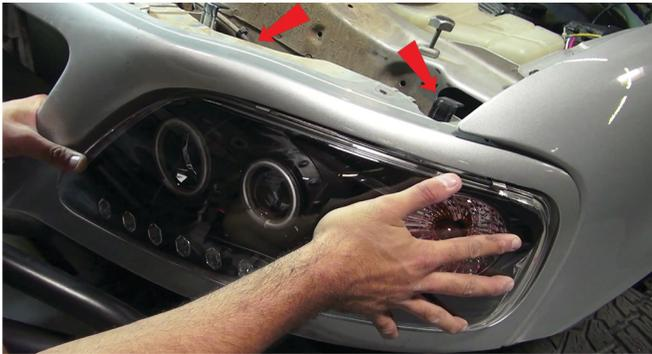
7) Push down on the two headlight retainer tabs.
