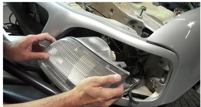
4) Unseat the headlight by pulling it forward, then remove the headlight socket. Then set the headlight aside.
