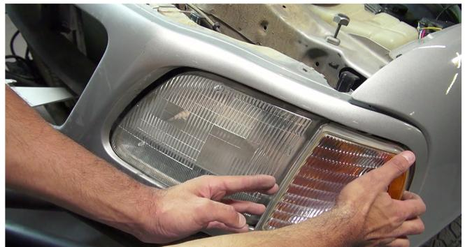
2) Pry out the corner lamp, then remove the turn signal socket and remove the corner lamp assembly and set it aside.
