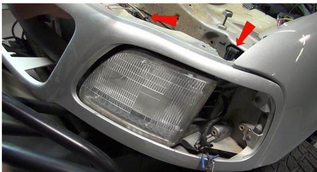
3) Pull the two headlight retainer tabs UP to release the headlight.
