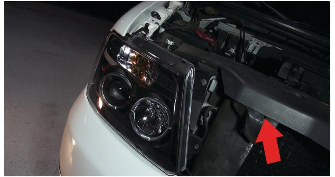
6) Replace the radiator shroud weatherstrip, then reinstall the plastic phillips head clip securing it, then close the hood.
