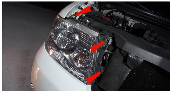
2) Peel back the radiator shroud weatherstrip. Remove the three 10mm bolts securing the headlight.
