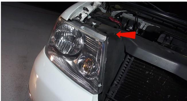
1) Open the hood. Remove the Phillips head clip securing the rubber radiator shroud weatherstrip.
