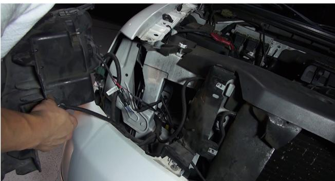
3) Unseat the headlight and remove the turn signal bulb sockets and disconnect the headlight wiring harness.
