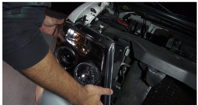
4) Locate the SPYDER headlight. Install turn signal bulb socket into SPYDER headlight, then connect the SPYDER headlight to the OEM headlight wiring harness.
