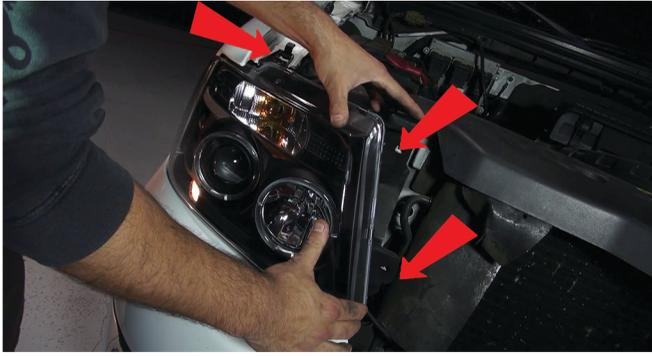
5) Seat the SPYDER headlight. Reinstall the three 10mm bolts securing the headlight.
