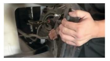
5) Disconnect the headlight bulb wiring harness and turn signal bulb.
