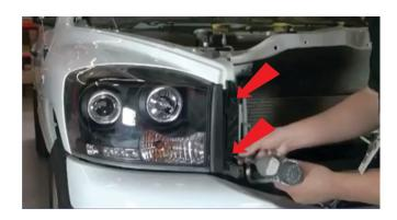
10) Reinstall the two T-25 Torx Screws securing the headlight.
