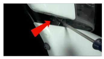
3) Using the access hole in the fender well, use a 10mm socket to remove the 10mm nut securing the headlight from behind, indicated here.
