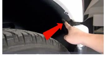
2) Move to the wheel well and remove the rubber access plug indicated.
