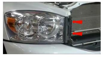
1) Open the hood. Remove the two T25 Torx screws securing the headlight.
