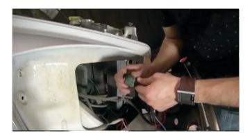
8) Connect the wiring harness from the SPYDER headlight to the OEM headlight harness.
