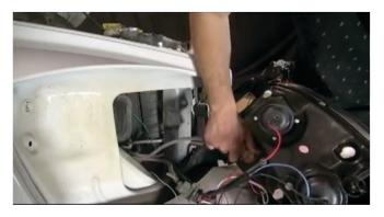
6) Locate your SPYDER headlight. Reinstall the turn signal bulb/socket into the SPYDER headlight housing by twisting it into place. Take care to ensure all bulb socket gaskets are in place and all vent hoses face down to prevent condensation.
