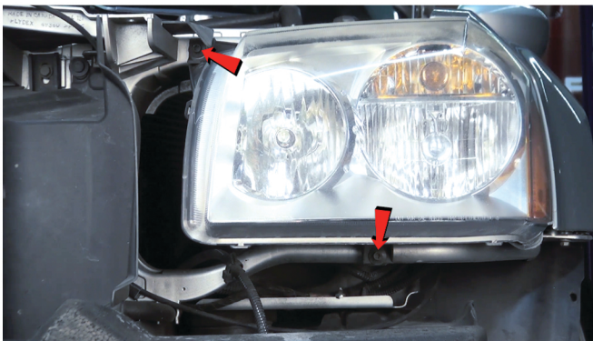
7) Remove [2x] T-30 torx screws securing the headlight.
