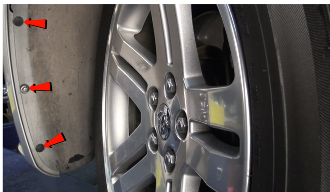
3) Remove [3x] plastic retainers securing the fender liner.
