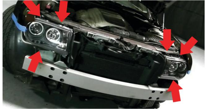
8) Time to replace the head lights. Seat the head lights back into position by lining up the brackets to the mounting holes. Use the 10mm socket to fasten the 10mm bolts back. There should be (3) per side.
