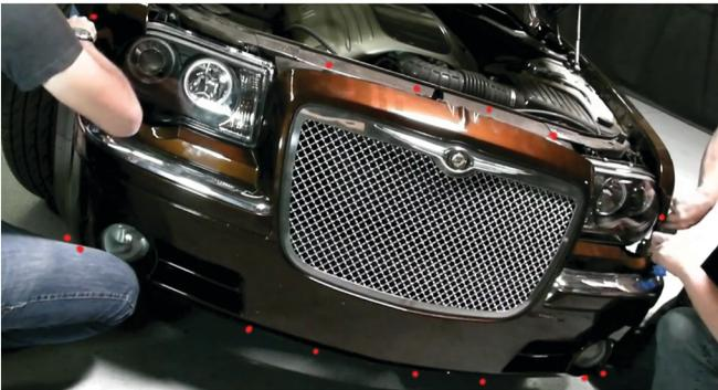
9) Place the bumper back by lining up the grill and corners with there mounting holes. You will need to replace the (4) clips on the grill, the 10 mm bolts on both bumper corners, (4) clips on both sides of the fender liners and (8) 8mm bolts on the bottom to secure the bumper back in place.
