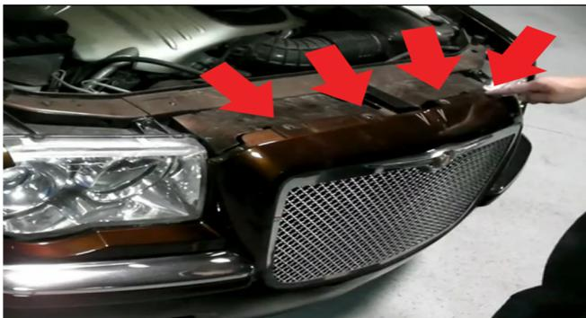
1) The bumper will need to be removed to install your new Spyder head lights. First you will start by removing the top (4) clips from the grill area. Using the Panel Popper pry the (4) clips from their mounting holes.
