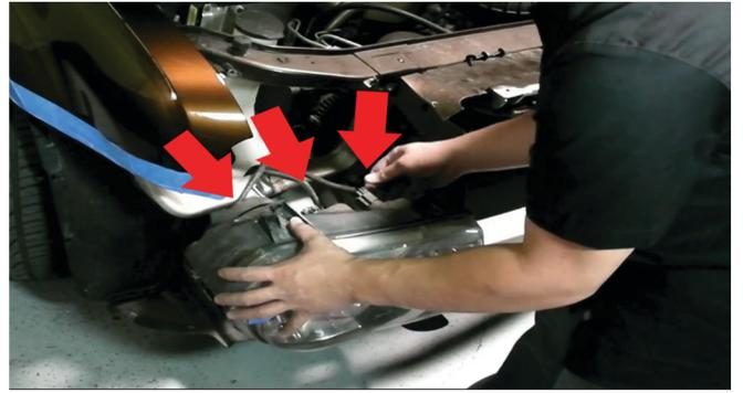
6) Next, you will need to remove the head light from the vehicle. Before it can be removed there are three sockets that are connected to the back of the head light. Twist these counter clockwise until they click.
