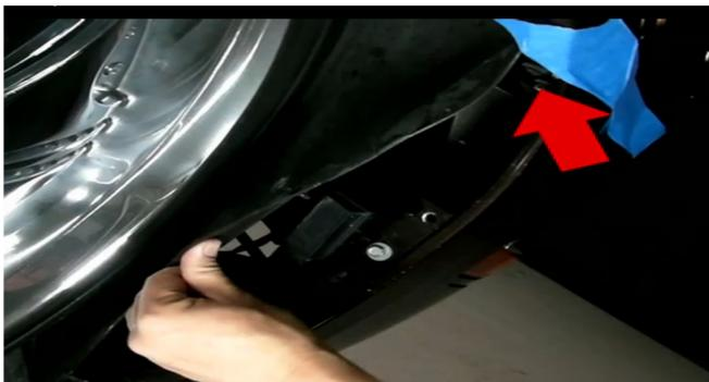
3) Next you will need to remove the 10mm bolt that is secured behind the fender liner. Use the 10mm socket or wrench to unscrew it from its bolt hole. Clips and bolts will need to be removed from both sides of the bumper.
