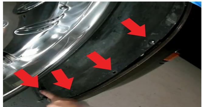
2) Next, detaching the fender liner from the bumper. Using the Panel Popper pry the (4) plastic fasteners from their mounting holes.
