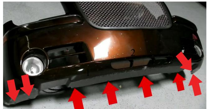
4) Before the bumper can be fully removed it will need to be detached from the slash guard. This is secured by (4) 8mm bolt on the outer edges of the bumper and (4) 8mm bolts on the inner portion. You will need to use the 8mm socket or wrench to remove these from there bolt holes.
