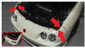
8) Next, seat the bumper, lining up the mount holes with their bolt holes. Replace the (4) 10mm bolts, one on top and another on the side to both sides. Next replace the (9) screws on the grill area to bolt down the mount plat and bumper.
