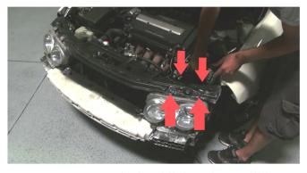
4) Now to remove the head lights, there will be (2) 10mm bolts behind the head light and (9) 10mm bolts on the top. Remove these and set them aside with the others. Untwist the Hi and Low beam bulbs from your OE head lights, set the head light aside.
