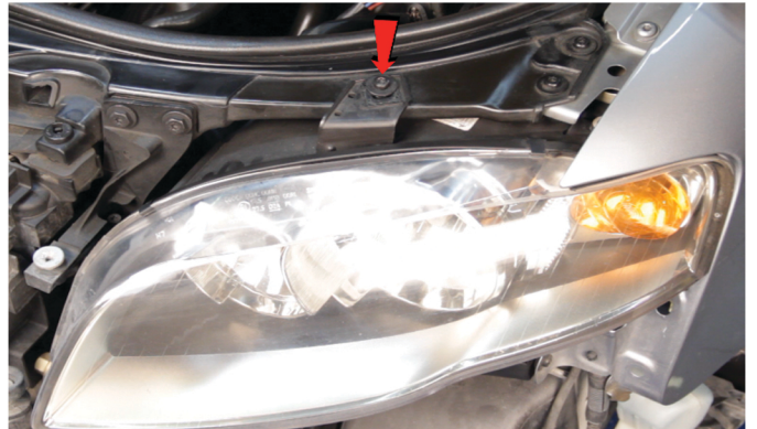
12) Remove [1x] T-30 torx screw securing the headlight.
