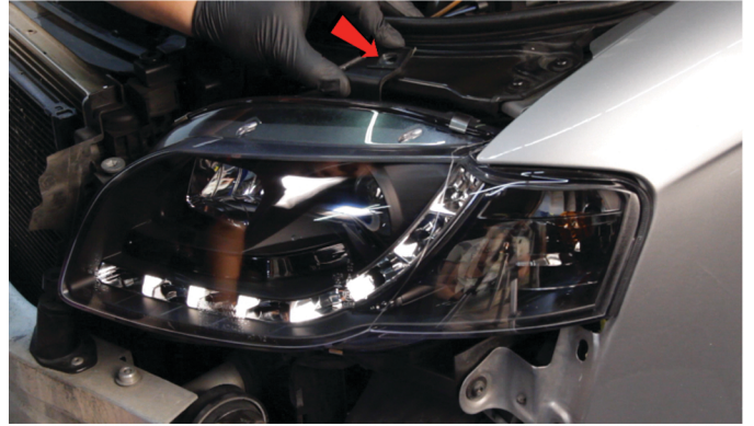
18) Install the included washer underneath the upper headlight tab.
