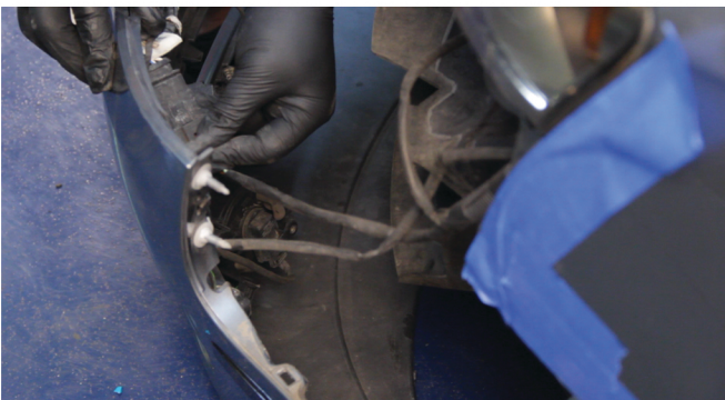
21) Reconnect the fog light and sidemarker master disconnects on the driver's side.
