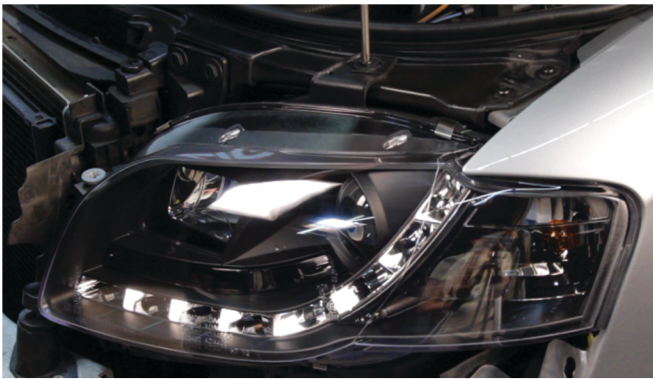
19) Reinstall [1x] T-30 torx screw.
