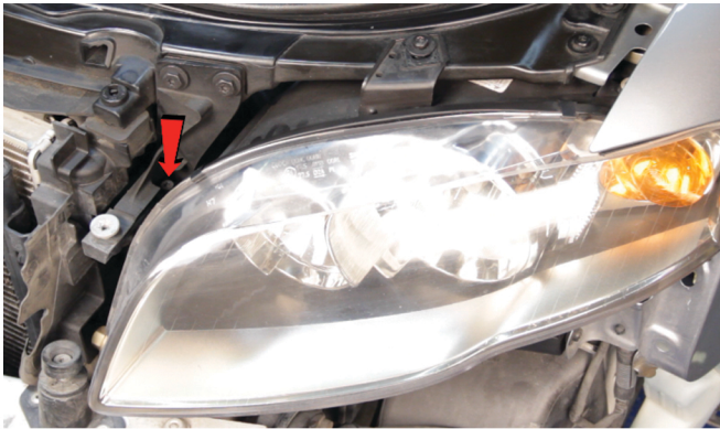
11) Loosen [1x] T-30 torx Screw. Loosen, but do not remove this screw.
