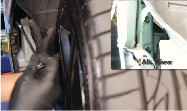
23) Reinstall [2x] 10mm bolts that secure the fascia to the fender.
