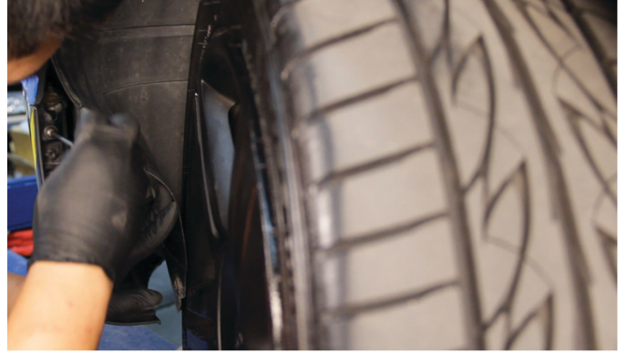
24) Reinstall [2x] T-25 torx screws to secure the fascia to the fender.
