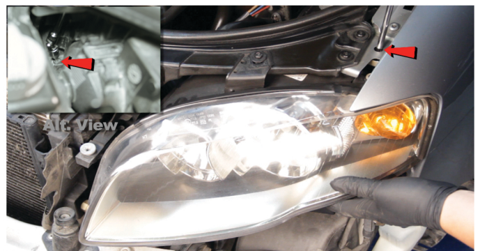
10) Loosen [1x] T-30 torx screw hidden underneath the core support using a long torx driver to loosen it through the access hole in the fender. Loosen, but do not completely remove this screw.
