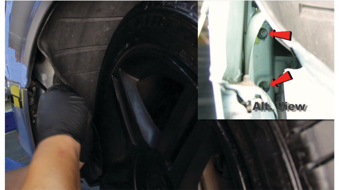
6) Peel back the fender liner for access, then remove [2x] 10mm nuts securing the fascia hidden deep inside the fender.
