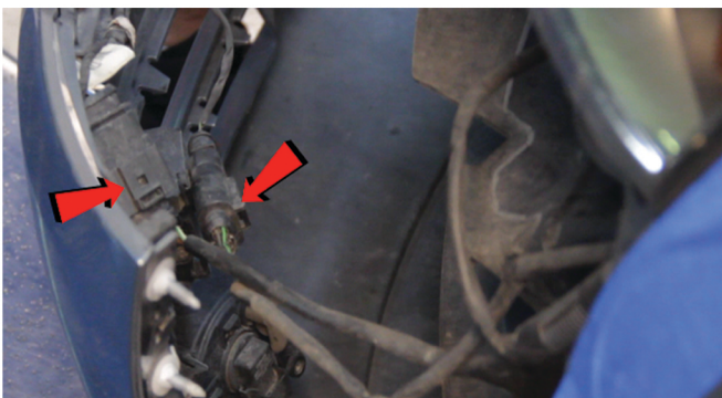
9) Disconnect the sidemarker and fog lamp master disconnects on the driver's side.
