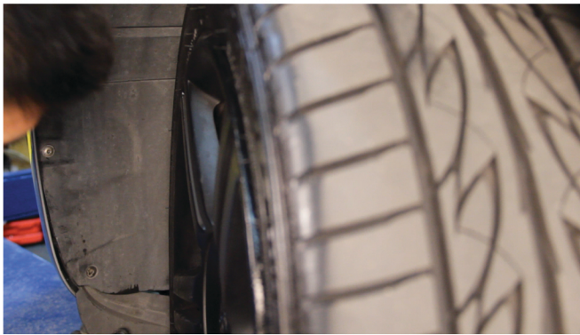
25) Reinstall [1x] T-25 torx screw to secure the fender liner.
