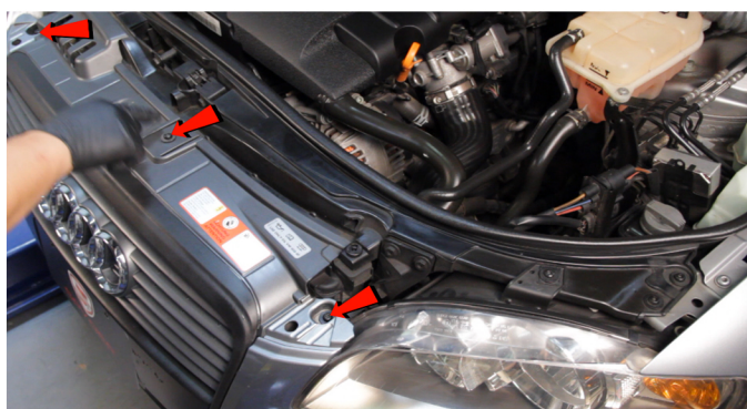
2) Remove [3x] T-30 Torx screws securing the fascia above the grille.
