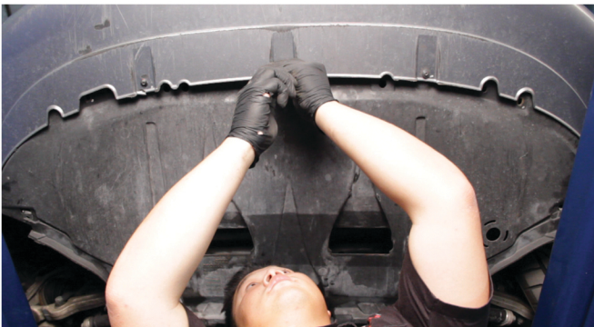
27) Reinstall [3x] T-25 torx screws to secure the fascia to the undertray.
