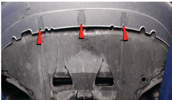
7) Remove [3x] T-25 torx screws securing the fascia to the undertray.
