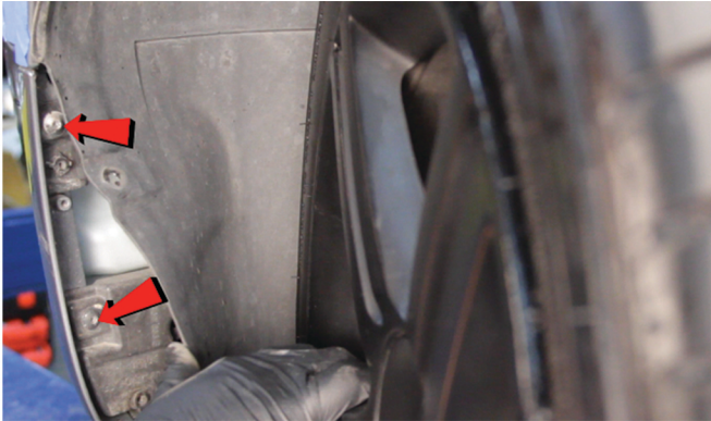
5) Remove [2x] T-25 torx screws securing the fascia to the fender.
