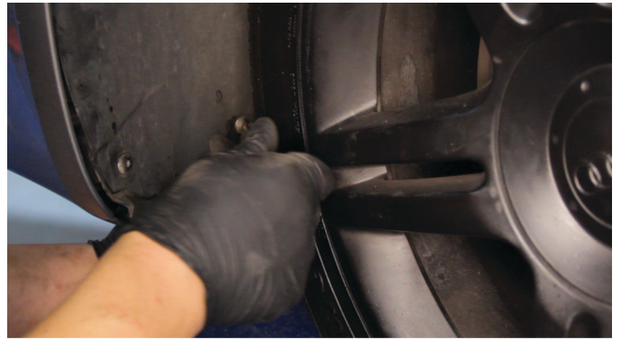
26) Seat the forward mudflap, then reinstall [2x] T-25 torx screws to secure the fender liner.
