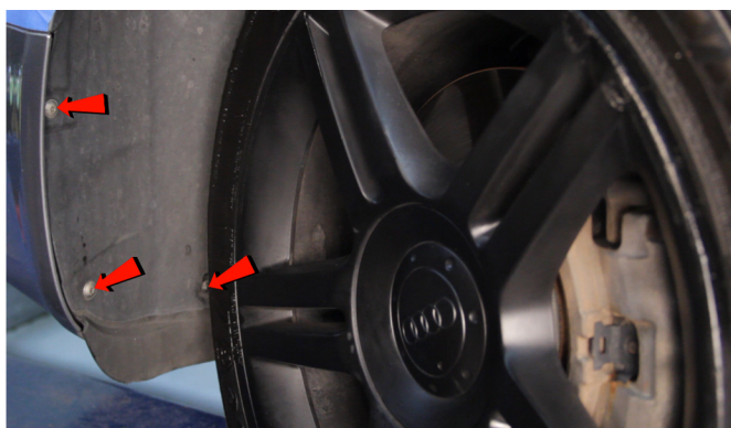
3) Remove [3x] T-25 Torx screws that secure the fender liner and the forward mudflap.
