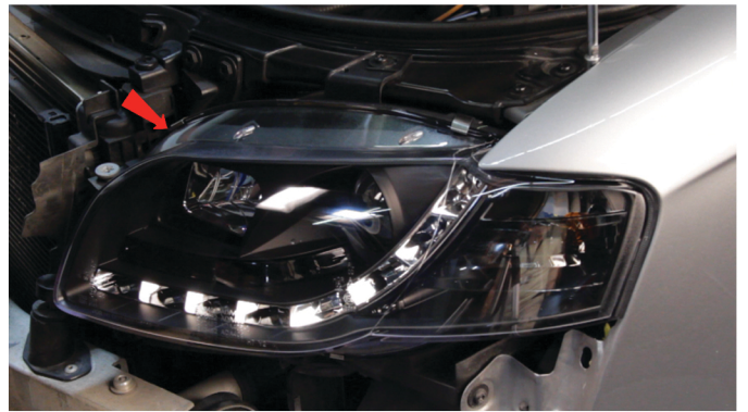
20) Tighten [2x] T-30 torx screws, the one hidden under the core support using a long torx driver through the access hole in the fender as well as the inboard one.
